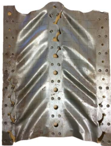
Figure 10.4.5: A photograph of shear buckling of a plate representing the damage pattern on the ship's hull inflicted upon grounding.
