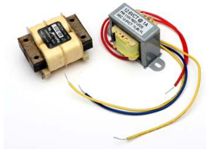
Figure 10.4.1 : Transformers suitable for consumer electronics devices. The unit on the left features four separate coils for enhanced flexibility.
