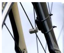
Figure 10.2.4 : Bicycle computer sensor and magnet.
