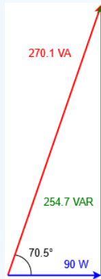
Figure 7.3.3: Power triangle for the circuit of Figure 7.3.2.
