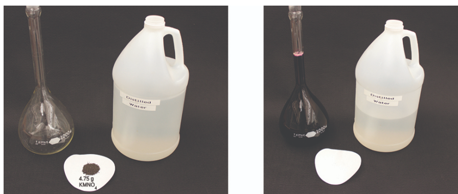
Figure 1.5.3: A solution of KMnO_4 is prepared by mixing water with 4.74 g of KMnO_4 in a flask. (credit: modification of work by Mark Ott)
