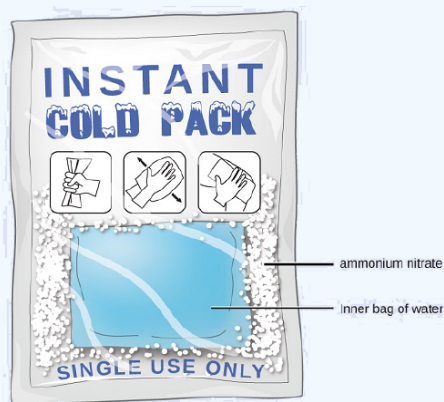
Figure 3.3.5 An instant cold pack consists of a bag containing solid ammonium nitrate and a second bag of water. When the bag of water is broken, the pack becomes cold because the dissolution of ammonium nitrate is an endothermic process that removes thermal energy from the water. The cold pack then removes thermal energy from your body.
