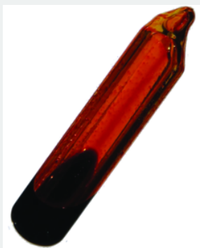
Figure 2.2.4: An equilibrium is pictured between liquid bromine, \text{Br}_2(\text{l}) , the dark liquid, and bromine vapor, \text{Br}_2(\text{g}) , the orange gas. Because the container is sealed, bromine vapor cannot escape and equilibrium is maintained. (credit: http://images-of-elements.com/bromine.php ).
