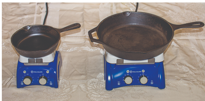
Figure 3.2.7: Due to its larger mass, a large frying pan has a larger heat capacity than a small frying pan. Because they are made of the same material, both frying pans have the same specific heat. (credit: Mark Blaser).
