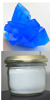
Figure 8.1.1: (left) Crystals of \text{CuSO}_4 \cdot 5\text{H}_2\text{O} . from Stephanb (via Wikipedia). (right) Anhydrous \text{CuSO}_4 after the water was removed.
