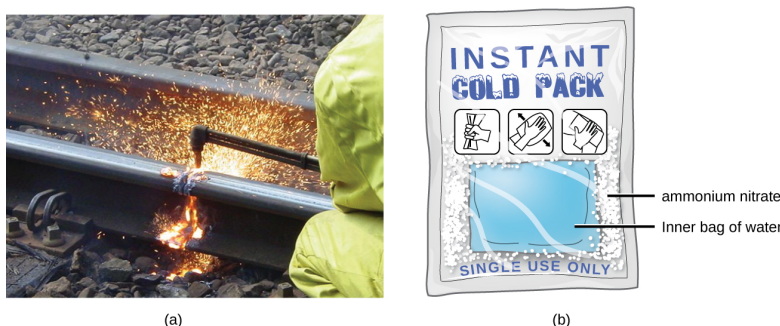
Figure 3.2.6: (a) An oxyacetylene torch produces heat by the combustion of acetylene in oxygen. The energy released by this exothermic reaction heats and then melts the metal being cut. The sparks are tiny bits of the molten metal flying away. (b) A cold pack uses an endothermic process to create the sensation of cold. (credit a: modification of work by “Skatebiker”/Wikimedia commons).
