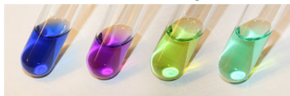
Figure 8.1.4: Color of various Ni(II) complexes in aqueous solution. From left to right, hexaamminenickel(II), tris(ethylenediamine)nickel(II), tetrachloronickelate(II) and hexaaquanickel(II). from LHcheM (via Wikipedia)
