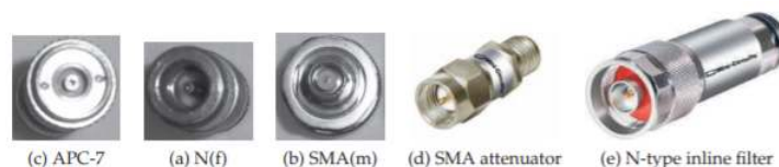
Figure 2.2.4: Various coaxial 50 \Omega transmission line connectors: (a) APC-7 coaxial connector ( 7 \text{ mm} outer conductor diameter); (b) female N-type (N(f)) coaxial connector ( 7 \text{ mm} ); (c) male SMA-type (SMA(m)) coaxial connector ( 3.5 \text{ mm} ); (d) DC to 26 \text{ GHz} , 2-W SMA precision fixed attenuator; and (e) N-type inline 500 \text{ MHz} lowpass filter. ((d) and (e) copyright 2012 Scientific Components Corporation d/b/a Mini-Circuits, used with permission [4]).
