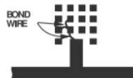
Figure 2.4.4: Open-circuited stub with variable length realized using wire bonding from the fixed stub to one of the bond pads. The bond pads are on the same layer as the strip metal layer and bonding to them extends the length of the open-circuited stub.
