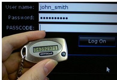
Figure 2.3.3.1: A disconnected token. The number must be copied into the PASSCODE field by hand. ("Disconnected Token" by Multiple Contributors, Wikipedia is licensed under CC BY-SA 3.0)
