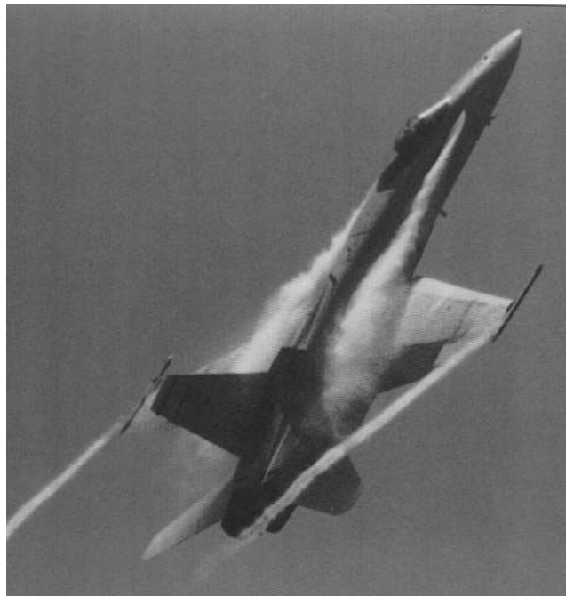
Figure 3.19: Vortex Flows on an F-18 (NASA Photo)
