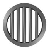
Figure 7.8.3: wire grid polarizer
