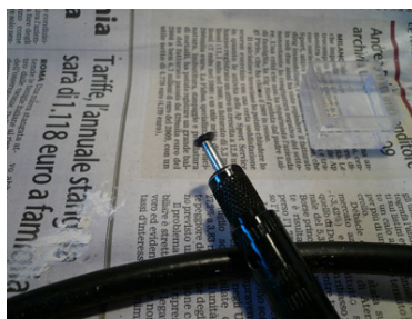
Figure 17.3.12: The tool made from a steel nailhead, mounted on a flex shaft.
