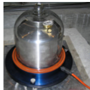
Figure 6. Housed in a vacuum under a protective dome inside a vault in the Santa Catalina Mountains north of Tucson, a seismometer similar to this one (which is located in Antarctica) registered the Nepal earthquake 15 minutes after the ground started shaking in the Himalayas.
