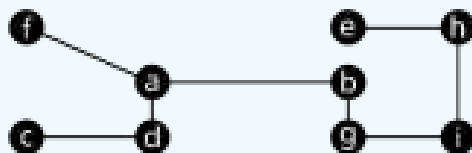
Figure 7.4.16 : Spanning Tree Formed Removing ac , cf , and be
