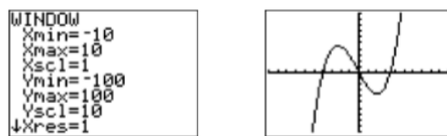
Figure 6.4.6: Adjusting the view so that the turning points of the polynomial are visible.
