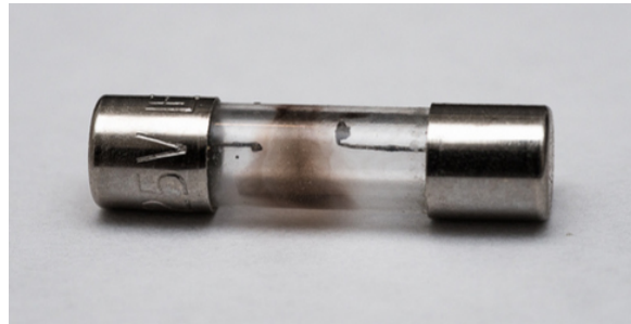
Figure 5.6.3: A fuse consists of a piece of wire between two contacts. When a current passes through the wire that is greater than the rated current, the wire melts, breaking the connection. Pictured is a “blown” fuse where the wire broke protecting a circuit (credit: modification of work by “Shardayy”/Flickr).
