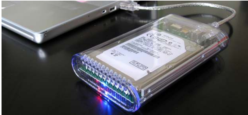
Figure [Math Processing Error] : An external hard drive attached to a computer works by magnetically encoding information that can be stored or retrieved quickly. A key idea in the development of digital devices is the ability to produce and use magnetic fields in this way. (credit: modification of work by “Miss Karen”/Flickr)
