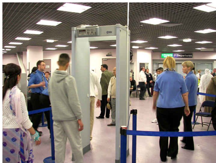
Figure 9.10.5: The familiar security gate at an airport not only detects metals, but can also indicate their approximate height above the floor. (credit: "Alexbuidrs"/Wikimedia Commons)
