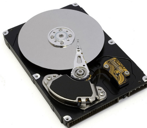
Figure 8.6.6: The inside of a hard disk drive. The silver disk contains the information, whereas the thin stylus on top of the disk reads and writes information to the disk.
