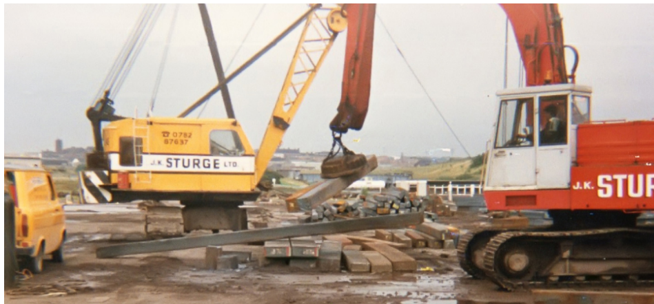
Figure 7.1.1: An industrial electromagnet is capable of lifting thousands of pounds of metallic waste. (credit: modification of work by "BedfordAI"/Flickr)
