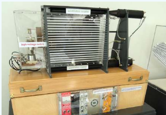
Figure 3.3.5: A spark chamber is used to trace the paths of high-energy particles. Ionization created by the particles as they pass through the gas between the plates allows a spark to jump. The sparks are perpendicular to the plates, following electric field lines between them. The potential difference between adjacent plates is not high enough to cause sparks without the ionization produced by particles from accelerator experiments (or cosmic rays). This form of detector is now archaic and no longer in use except for demonstration purposes. (credit b: modification of work by Jack Collins)
