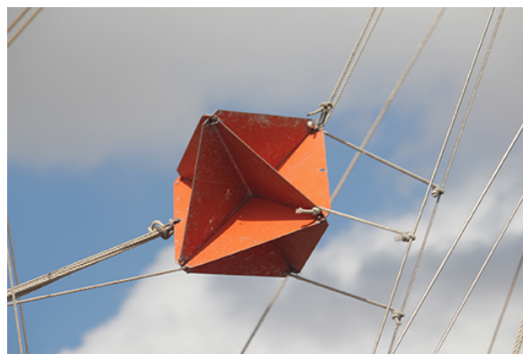
Figure 11.5.7: A radar reflector hoisted on a sailboat is a type of corner reflector. (credit: Tim Sheerman-Chase)
