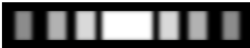
Figure 13.3.3: (a) The calculated intensity distribution of a single-slit diffraction pattern. (b) The actual diffraction pattern.
