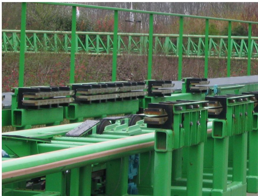
Figure 9.6.7: The rows of rare-earth magnets (protruding horizontally) are used for magnetic braking in roller coasters. (credit: Stefan Scheer)
