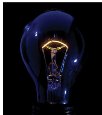
Figure 5.3.3: The incandescent lamp is a simple design. A tungsten filament is placed in a partially evacuated glass envelope. One end of the filament is attached to the screw base, which is made out of a conducting material. The second end of the filament is attached to a second contact in the base of the bulb. The two contacts are separated by an insulating material. Current flows through the filament, and the temperature of the filament becomes large enough to cause the filament to glow and produce light. However, these bulbs are not very energy efficient, as evident from the heat coming from the bulb. In the year 2012, the United States, along with many other countries, began to phase out incandescent lamps in favor of more energy-efficient lamps, such as light-emitting diode (LED) lamps and compact fluorescent lamps (CFL) (credit right: modification of work by Serge Saint).
