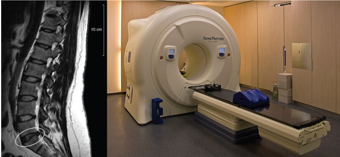
Figure 5.1.1: Magnetic resonance imaging (MRI) uses superconducting magnets and produces high-resolution images without the danger of radiation. The image on the left shows the spacing of vertebrae along a human spinal column, with the circle indicating where the vertebrae are too close due to a ruptured disc. On the right is a picture of the MRI instrument, which surrounds the patient on all sides. A large amount of electrical current is required to operate the electromagnets (credit right: modification of work by "digital cat"/Flickr).
