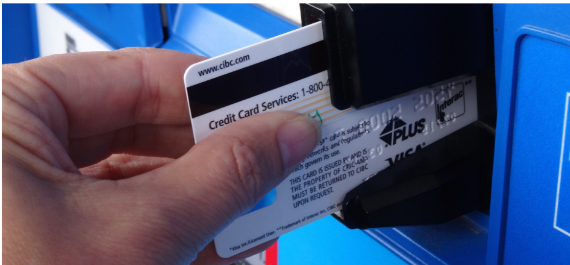
Figure 9.1.1: The black strip found on the back of credit cards and driver's licenses is a very thin layer of magnetic material with information stored on it. Reading and writing the information on the credit card is done with a swiping motion. The physical reason why this is necessary is called electromagnetic induction and is discussed in this chapter.
