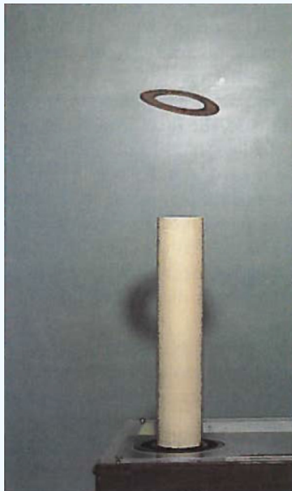
Figure 9.3.4: The jumping ring. When a current is turned on in the vertical solenoid, a current is induced in the metal ring. The stray field produced by the solenoid causes the ring to jump off the solenoid.
