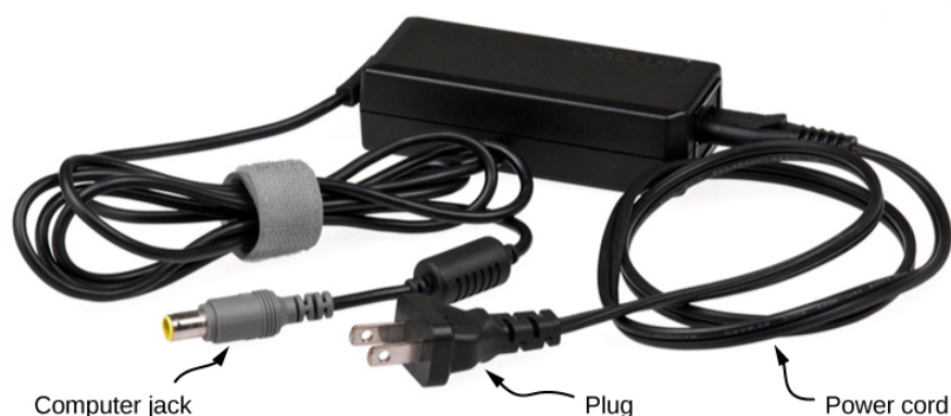
Figure 1.3.1: This power adapter uses metal wires and connectors to conduct electricity from the wall socket to a laptop computer. The conducting wires allow electrons to move freely through the cables, which are shielded by rubber and plastic. These materials act as insulators that don't allow electric charge to escape outward. (credit: modification of work by "Evan-Amos"/Wikimedia Commons)
