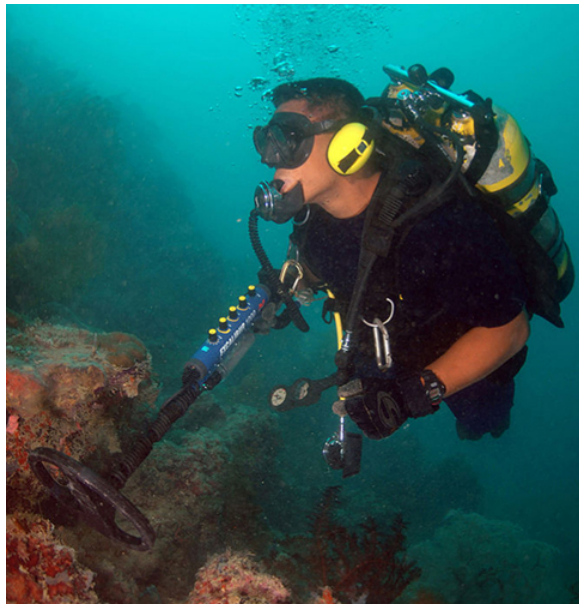
Figure 10.6.3: When a metal detector comes near a piece of metal, the self-inductance of one of its coils changes. This causes a shift in the resonant frequency of a circuit containing the coil. That shift is detected by the circuitry and transmitted to the diver by means of the headphones.
