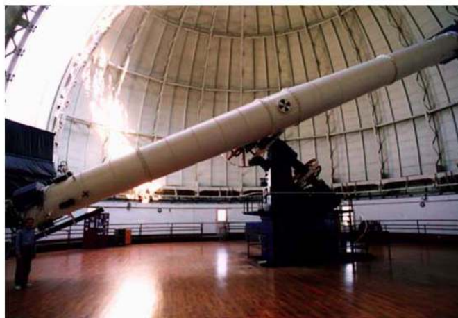
Figure 11.10.9.6: In 1897, the Yerkes Observatory in Wisconsin (USA) built a large refracting telescope with an objective lens that is 40 inches in diameter and has a tube length of 62 feet. (credit: Yerkes Observatory, University of Chicago)
