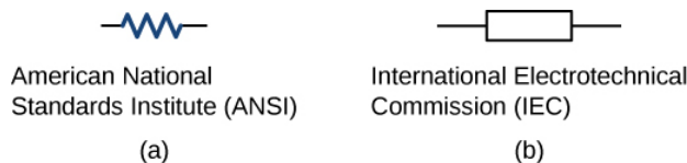
Figure 5.4.2: Symbols for a resistor used in circuit diagrams. (a) The ANSI symbol; (b) the IEC symbol.
