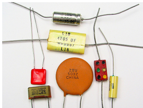
Figure 4.2.3: These are some typical capacitors used in electronic devices. A capacitor's size is not necessarily related to its capacitance value.
