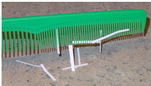
Figure 1.2.2: After being used to comb hair, this comb attracts small strips of paper from a distance, without physical contact. Investigation of this behavior helped lead to the concept of the electric force.
