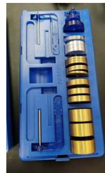
Figure 2.1: Pulley hangers (left) / Mass (right side top to bottom): 0.5g, 1g, 2g, 5g, 10g, 20g, 50g, 100g :
