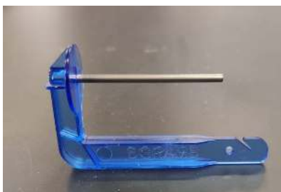
Figure 2.1: Pulley hanger: This object has a mass of 5 grams, so consider that when calculating.
