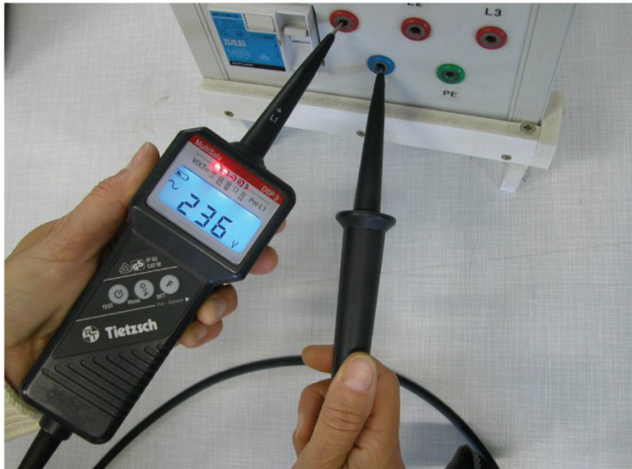
Figure 21.4.2: (a) To measure potential differences in this series circuit, the voltmeter (V) is placed in parallel with the voltage source or either of the resistors. Note that terminal voltage is measured between points a and b. It is not possible to connect the voltmeter directly across the emf without including its internal resistance r (b) A digital voltmeter in use. (credit: Messtechniker, Wikimedia Commons)
