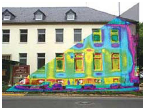
Figure 14.7.5: A thermograph of part of a building shows temperature variations, indicating where heat transfer to the outside is most severe. Windows are a major region of heat transfer to the outside of homes. (credit: U.S. Army)
