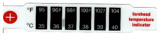
Figure 13.1.2: Each of the six squares on this plastic (liquid crystal) thermometer contains a film of a different heat-sensitive liquid crystal material. Below 95^{\circ} F all six squares are black. When the plastic thermometer is exposed to temperature that increases to 95^{\circ} F the first liquid crystal square changes color. When the temperature increases above 96.8^{\circ} F the second liquid crystal square also changes color, and so forth. (credit: Arkkrishna, Wikimedia Commons)
