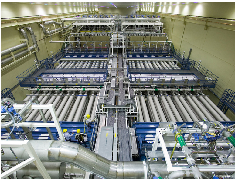
Figure 32.5.9: National Ignition Facility (CA). This image shows a laser bay where 192 laser beams will focus onto a small D-T target, producing fusion. (credit: Lawrence Livermore National Laboratory, Lawrence Livermore National Security, LLC, and the Department of Energy)
