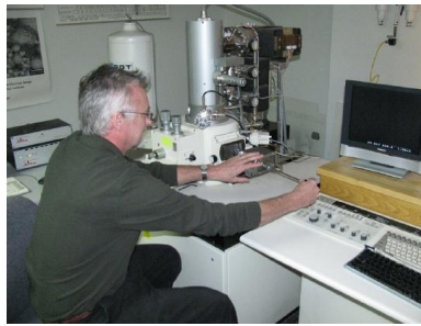
Figure 26.4.7: An electron microscope has the capability to image individual atoms on a material. The microscope uses vacuum technology, sophisticated detectors and state of the art image processing software. (credit: Dave Pape)
