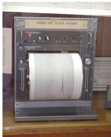
A seismograph as described in above problem.(credit: Oleg Alexandrov)
