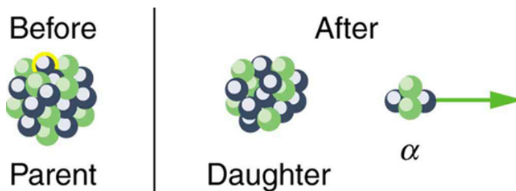
Figure 31.4.2: Alpha decay is the separation of a {}^4\text{He} nucleus from the parent. The daughter nucleus has two fewer protons and two fewer neutrons than the parent. Alpha decay occurs spontaneously only if the daughter and {}^4\text{He} nucleus have less total mass than the parent.
