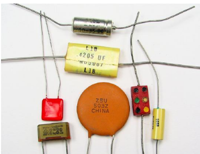
Figure 19.5.3: Some typical capacitors. Size and value of capacitance are not necessarily related. (credit: Windell Oskay)
