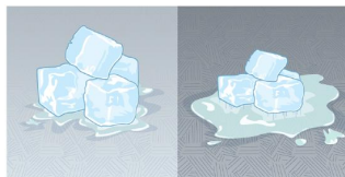
Figure 14.7.3: This illustration shows that the darker pavement is hotter than the lighter pavement (much more of the ice on the right has melted), although both have been in the sunlight for the same time. The thermal conductivities of the pavements are the same.
