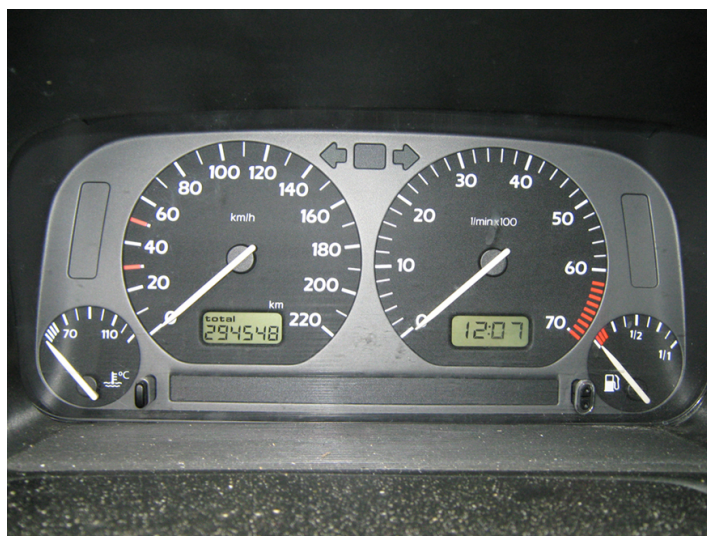
Figure 21.4.1: The fuel and temperature gauges (far right and far left, respectively) in this 1996 Volkswagen are voltmeters that register the voltage output of “sender” units, which are hopefully proportional to the amount of gasoline in the tank and the engine temperature. (credit: Christian Giersing)
