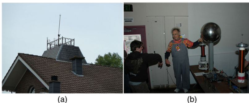
Figure 18.7.8: (a) A lightning rod is pointed to facilitate the transfer of charge. (credit: Romaine, Wikimedia Commons) (b) This Van de Graaff generator has a smooth surface with a large radius of curvature to prevent the transfer of charge and allow a large voltage to be generated. The mutual repulsion of like charges is evident in the person’s hair while touching the metal sphere. (credit: Jon ‘ShakataGaNai’ Davis/Wikimedia Commons).
