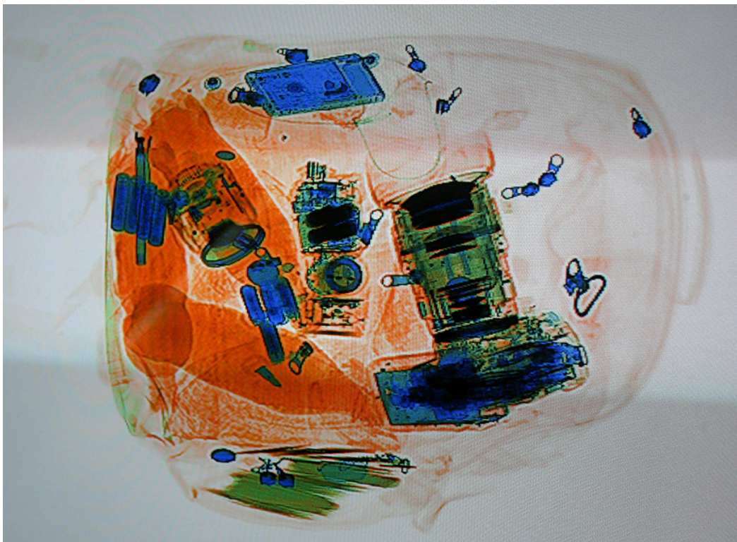
Figure 30.4.5: This x-ray image shows the contents of a piece of luggage. The denser the material, the darker the shadow. (credit: IDuke, Wikimedia Commons)
