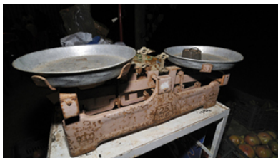
Figure 1.3.1: A double-pan mechanical balance is used to compare different masses. Usually an object with unknown mass is placed in one pan and objects of known mass are placed in the other pan. When the bar that connects the two pans is horizontal, then the masses in both pans are equal. The “known masses” are typically metal cylinders of standard mass such as 1 gram, 10 grams, and 100 grams. (credit: Serge Melki)
