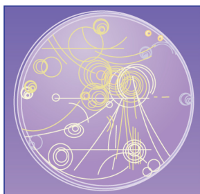
Figure 22.5.1: Trails of bubbles are produced by high-energy charged particles moving through the superheated liquid hydrogen in this artist's rendition of a bubble chamber. There is a strong magnetic field perpendicular to the page that causes the curved paths of the particles. The radius of the path can be used to find the mass, charge, and energy of the particle.
