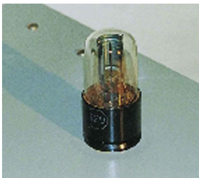
Figure 29.2.1: The photoelectric effect can be observed by allowing light to fall on the metal plate in this evacuated tube. Electrons ejected by the light are collected on the collector wire and measured as a current. A retarding voltage between the collector wire and plate can then be adjusted so as to determine the energy of the ejected electrons. For example, if it is sufficiently negative, no electrons will reach the wire. (credit: P.P. Urone)
