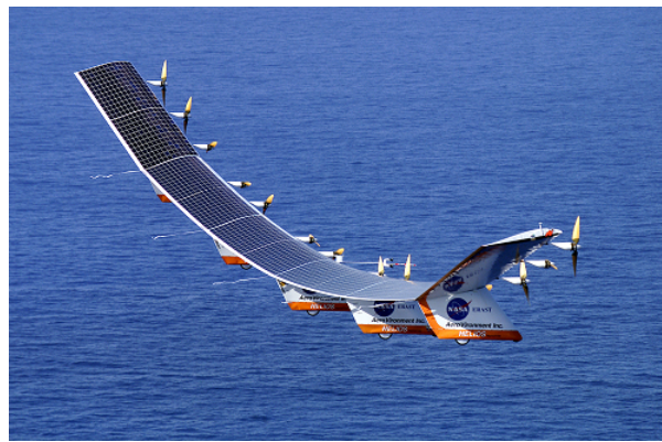
Figure 7.6.1: Solar energy is converted into electrical energy by solar cells, which is used to run a motor in this solar-power aircraft. (credit: NASA)
