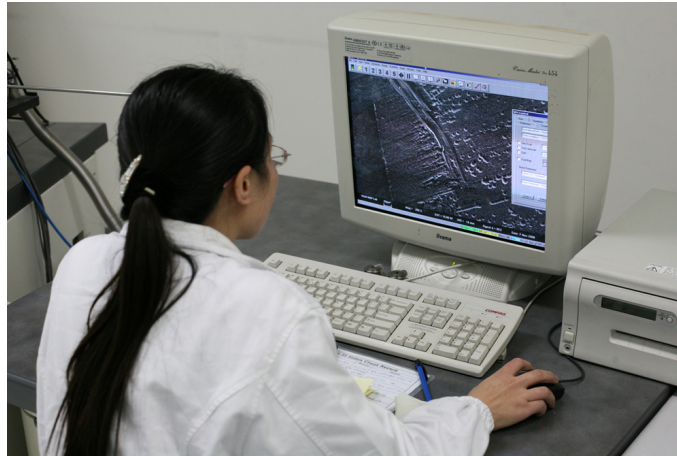
Figure 26.0.1: A scientist examines minute details on the surface of a disk drive at a magnification of 100,000 times. The image was produced using an electron microscope. (credit: Robert Scoble)
