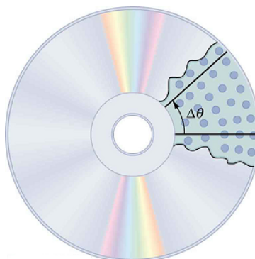
Figure 6.1.1: All points on a CD travel in circular arcs. The pits along a line from the center to the edge all move through the same angle \Delta\theta in a time \Delta t .
