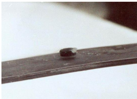
Figure 34.6.2: One characteristic of a superconductor is that it excludes magnetic flux and, thus, repels other magnets. The small magnet levitated above a high-temperature superconductor, which is cooled by liquid nitrogen, gives evidence that the material is superconducting. When the material warms and becomes conducting, magnetic flux can penetrate it, and the magnet will rest upon it. (credit: Saperaud)
