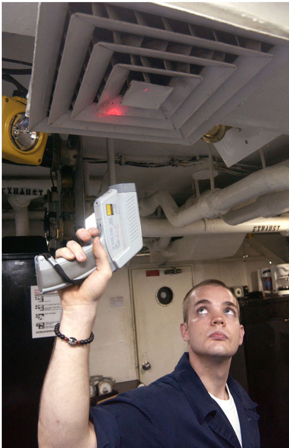
Figure 13.1.3: Fireman Jason Ormand uses a pyrometer to check the temperature of an aircraft carrier's ventilation system. Infrared radiation (whose emission varies with temperature) from the vent is measured and a temperature readout is quickly produced. Infrared measurements are also frequently used as a measure of body temperature. These modern thermometers, placed in the ear canal, are more accurate than alcohol thermometers placed under the tongue or in the armpit. (credit: Lamel J. Hinton/U.S. Navy)
