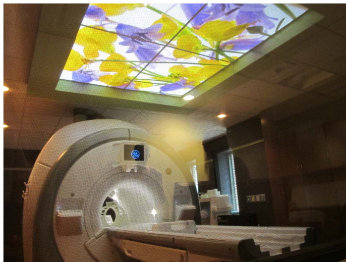
Figure 22.2.3: Instrument for magnetic resonance imaging (MRI). The device uses a superconducting cylindrical coil for the main magnetic field. The patient goes into this “tunnel” on the gurney. (credit: Bill McChesney, Flickr)
