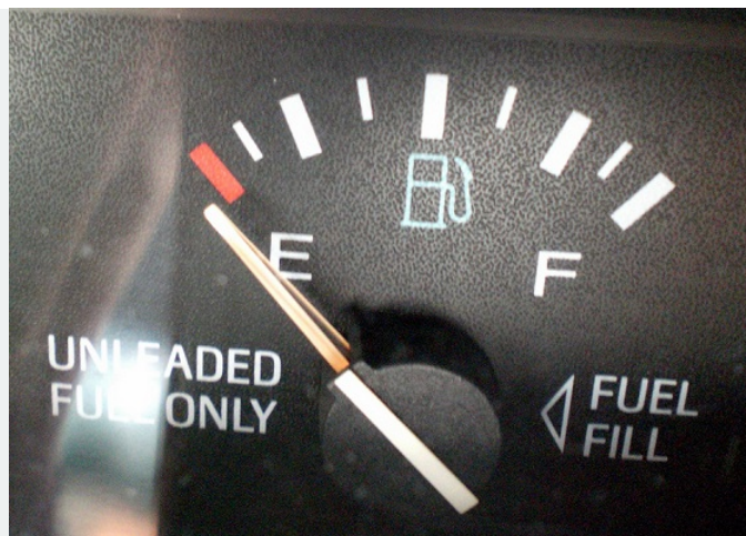
Figure 13.2.4: Because the gas expands more than the gas tank with increasing temperature, you can't drive as many miles on "empty" in the summer as you can in the winter. (credit: Hector Alejandro, Flickr)
