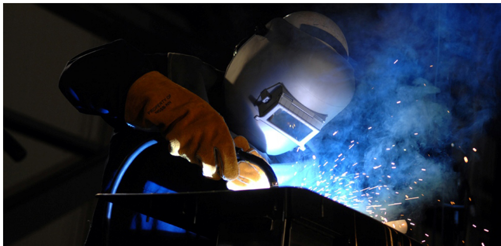
Figure 13.0.1: The welder's gloves and helmet protect him from the electric arc that transfers enough thermal energy to melt the rod, spray sparks, and burn the retina of an unprotected eye. The thermal energy can be felt on exposed skin a few meters away, and its light can be seen for kilometers. (credit: Kevin S. O'Brien/U.S. Navy)
