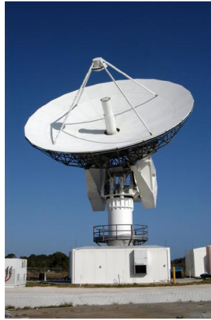
Figure 24.0.2: The electromagnetic waves sent and received by this 50-foot radar dish antenna at Kennedy Space Center in Florida are not visible, but help track expendable launch vehicles with high-definition imagery. The first use of this C-band radar dish was for the launch of the Atlas V rocket sending the New Horizons probe toward Pluto. (credit: NASA)
