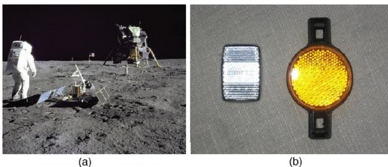
Figure 25.4.5: (a) Astronauts placed a corner reflector on the moon to measure its gradually increasing orbital distance. (credit: NASA) (b) The bright spots on these bicycle safety reflectors are reflections of the flash of the camera that took this picture on a dark night. (credit: Julo, Wikimedia Commons)
