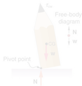
Figure 9.3.3: If the pencil is displaced slightly to the side (counterclockwise), it is no longer in equilibrium. Its weight produces a clockwise torque that returns the pencil to its equilibrium position.
