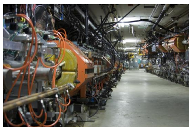
Figure 22.5.7: The Fermilab facility in Illinois has a large particle accelerator (the most powerful in the world until 2008) that employs magnetic fields (magnets seen here in orange) to contain and direct its beam. This and other accelerators have been in use for several decades and have allowed us to discover some of the laws underlying all matter. (credit: ammcgrim, Flickr)
