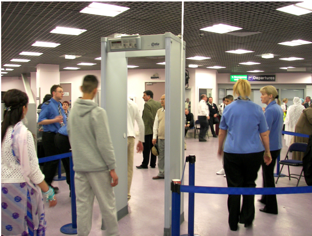
Figure 23.12.5: The familiar security gate at an airport can not only detect metals but also indicate their approximate height above the floor. (credit: Alexbuidrs, Wikimedia Commons)
