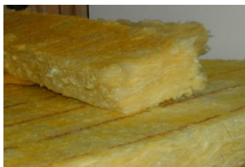
Figure 14.5.4: The fiberglass batt is used for insulation of walls and ceilings to prevent heat transfer between the inside of the building and the outside environment. (CC BY-SA 3.0; Radomil).
