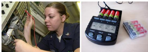
Figure 21.2.6: These two battery testers measure terminal voltage under a load to determine the condition of a battery. The large device is being used by a U.S. Navy electronics technician to test large batteries aboard the aircraft carrier USS Nimitz and has a small resistance that can dissipate large amounts of power. (credit: U.S. Navy photo by Photographer's Mate Airman Jason A. Johnston) The small device is used on small batteries and has a digital display to indicate the acceptability of their terminal voltage. (credit: Keith Williamson)
