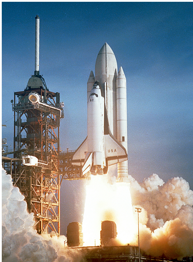
Figure 8.7.2: The space shuttle had a number of reusable parts. Solid fuel boosters on either side were recovered and refueled after each flight, and the entire orbiter returned to Earth for use in subsequent flights. The large liquid fuel tank was expended. The space shuttle was a complex assemblage of technologies, employing both solid and liquid fuel and pioneering ceramic tiles as reentry heat shields. As a result, it permitted multiple launches as opposed to single-use rockets. (credit: NASA)
