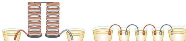
Figure 21.2.9: Batteries are multiple connections of individual cells, as shown in this modern rendition of an old print. Single cells, such as AA or C cells, are commonly called batteries, although this is technically incorrect.
