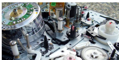
Figure 23.5.2: Recording and playback heads used with audio and video magnetic tapes. (credit: Steve Jurvetson)
