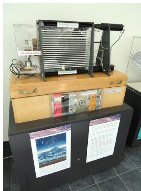
Figure 19.2.2: A spark chamber is used to trace the paths of high-energy particles. Ionization created by the particles as they pass through the gas between the plates allows a spark to jump. The sparks are perpendicular to the plates, following electric field lines between them. The potential difference between adjacent plates is not high enough to cause sparks without the ionization produced by particles from accelerator experiments (or cosmic rays). (credit: Daderot, Wikimedia Commons)
