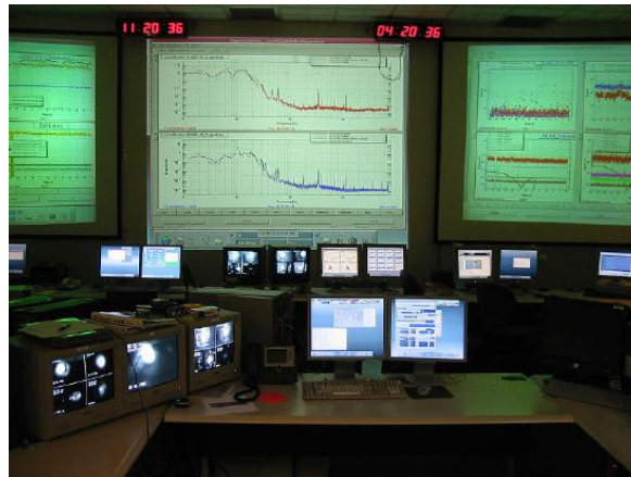
Figure 34.2.6: The control room of the LIGO gravitational wave detector. Gravitational waves will cause extremely small vibrations in a mass in this detector, which will be detected by laser interferometer techniques. Such detection in coincidence with other detectors and with astronomical events, such as supernovas, would provide direct evidence of gravitational waves. (credit: Tobin Fricke)
