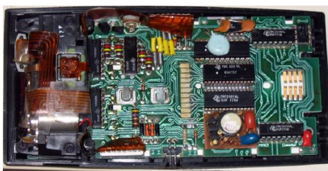
Figure 19.7.1: Energy stored in the large capacitor is used to preserve the memory of an electronic calculator when its batteries are charged. (credit: Kucharek, Wikimedia Commons)
