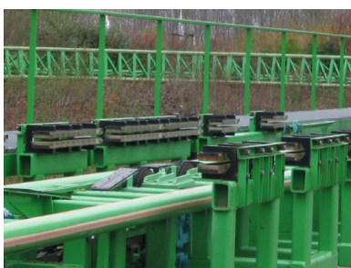
Figure 23.7.7: The rows of rare earth magnets (protruding horizontally) are used for magnetic braking in roller coasters. (credit: Stefan Scheer, Wikimedia Commons)
