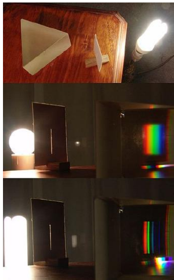
A simple spectroscope: A very simple spectroscope based on a prism
