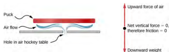
Figure 6.10.2: An air hockey table is useful in illustrating Newton's laws. When the air is off, friction quickly slows the puck; but when the air is on, it minimizes contact between the puck and the hockey table, and the puck glides far down the table.
