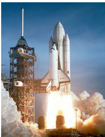
Figure 9.11.1: The space shuttle had a number of reusable parts. Solid fuel boosters on either side were recovered and refueled after each flight, and the entire orbiter returned to Earth for use in subsequent flights. The large liquid fuel tank was expended. The space shuttle was a complex assemblage of technologies, employing both solid and liquid fuel, and pioneering ceramic tiles as reentry heat shields. As a result, it permitted multiple launches as opposed to single-use rockets. (credit: modification of work by NASA)
