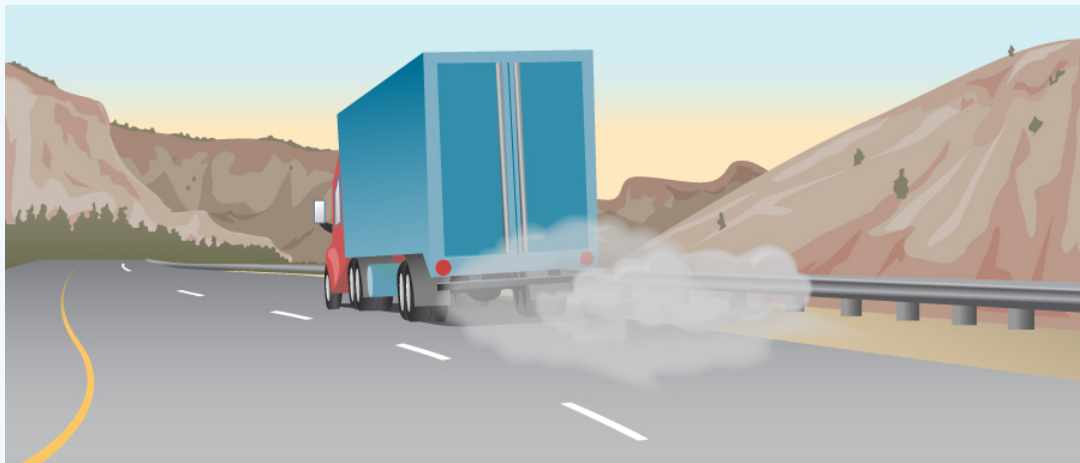
Figure 3: The smoking brakes on a braking truck are visible evidence of the mechanical equivalent of heat.
