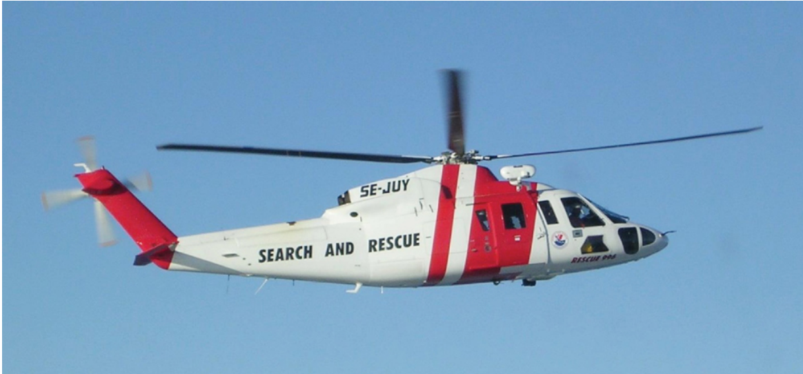
Figure 11.18.1: A helicopter has its main lift blades rotating to keep the aircraft airborne. Due to conservation of angular momentum, the body of the helicopter would want to rotate in the opposite sense to the blades, if it were not for the small rotor on the tail of the aircraft, which provides thrust to stabilize it.
