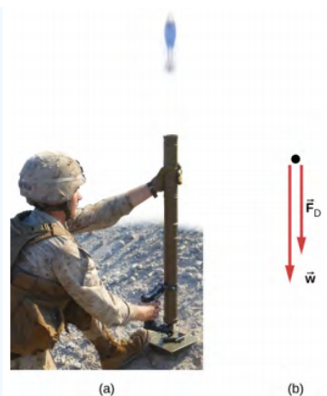
Figure 7.3.8: (a) The mortar fires a shell straight up; we consider the friction force provided by the air. (b) A free-body diagram is shown which indicates all the forces on the mortar shell.
