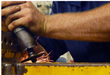
Figure 8.15.1: A grinding wheel applies a non-conservative force, because the work done depends on how many rotations the wheel makes, so it is path-dependent.
