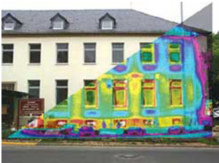
Figure 14: A thermograph of part of a building shows temperature variations, indicating where heat transfer to the outside is most severe. Windows are a major region of heat transfer to the outside of homes. (credit: US Army)
