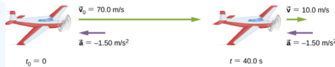
Figure 4.5.2: The airplane lands with an initial velocity of 70.0 m/s and slows to a final velocity of 10.0 m/s before heading for the terminal. Note the acceleration is negative because its direction is opposite to its velocity, which is positive.
