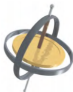
Figure 11.22.1: A gyroscope consists of a spinning disk about an axis that is free to assume any orientation.
