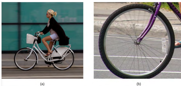
Figure 11.19.1: (a) The bicycle moves forward, and its tires do not slip. The bottom of the slightly deformed tire is at rest with respect to the road surface for a measurable amount of time. (b) This image shows that the top of a rolling wheel appears blurred by its motion, but the bottom of the wheel is instantaneously at rest. (credit a: modification of work by Nelson Lourenço; credit b: modification of work by Colin Rose)
