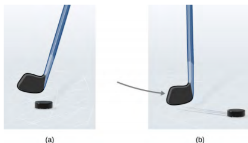
Figure 6.10.1: (a) A hockey puck is shown at rest; it remains at rest until an outside force such as a hockey stick changes its state of rest; (b) a hockey puck is shown in motion; it continues in motion in a straight line until an outside force causes it to change its state of motion. Although it is slick, an ice surface provides some friction that slows the puck.
