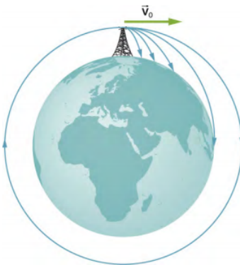
Figure 5.4.7: Projectile to satellite. In each case shown here, a projectile is launched from a very high tower to avoid air resistance. With increasing initial speed, the range increases and becomes longer than it would be on level ground because Earth curves away beneath its path. With a speed of 8000 m/s, orbit is achieved.
