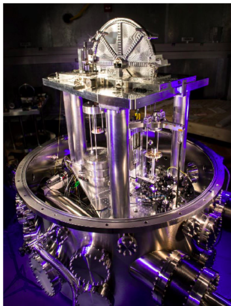
Figure 1.7.4: Redefining the SI unit of mass. The U.S. National Institute of Standards and Technology’s Kibble balance is a machine that balances the weight of a test mass with the resulting electrical current needed for a force to balance it.
