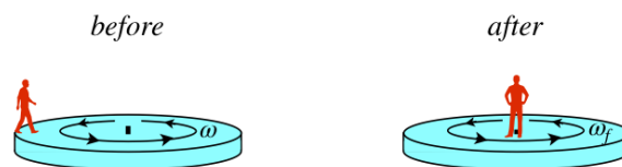
Figure 6.3.2 – System Changes Rotational Inertia While Rotating
