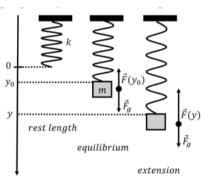
Figure 13.2.1: A vertical spring-mass system.
