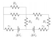
Figure 20.3.1: A circuit that can be simplified and then solved with Kirchoff's rules.
