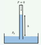
Figure 15.1.12: A Torricelli barometer.
