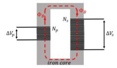
Figure 23.5.1: A transformer converts a primary alternating voltage,  $\Delta V_p$ , to a secondary alternating voltage,  $\Delta V_s$ . The magnetic flux produced in one coil is transmitted by an iron core to the secondary coil, where a different voltage is induced, depending on the ratio of the number of windings in each coil.
