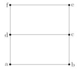
Figure 20.2.1: A circuit that has 3 loops and 2 junctions.
