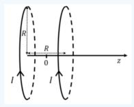
Figure 22.7.2: A Helmholtz coil arrangement.
