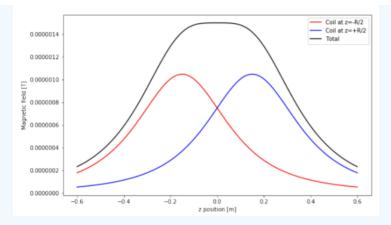
**Figure** 22.7.3 *Magnetic field from each coil, as well as their sum, for two coils in the Helmholtz configuration.* As advertised, we see a region between the Helmholtz coils where the magnetic field is nearly uniform.
