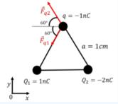
Figure 16.2.3: Force vectors on charge q.
