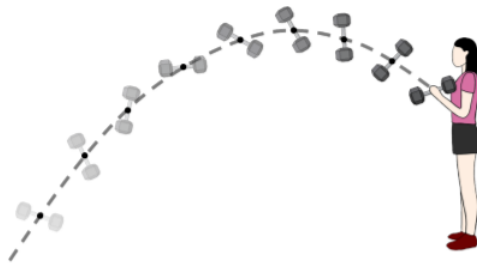
Figure 10.3.1: The motion of the center of mass of a dumbbell is described by Newton's Second Law, even if the motion of the rotating dumbbell is more complex.
