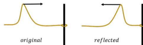
Figure 14.3.3: When the end of the rope is free, the reflected pulse will be upright.
