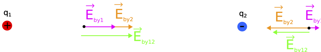
Figure 11.3.4: Net Electric Field by Multiple Point Charges (1D vector addition)
