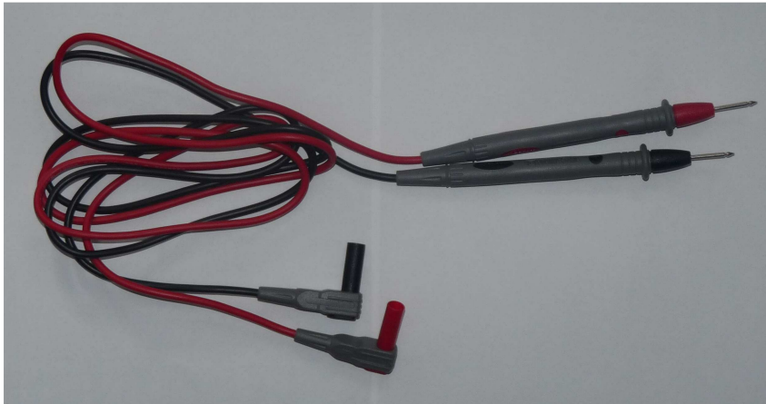
Figure 3.1.1: These leads used to connect test equipment to circuits in a laboratory are a very rudimentary form of transmission line, suitable only for very low frequencies. (Public Domain; Dmitry G)
