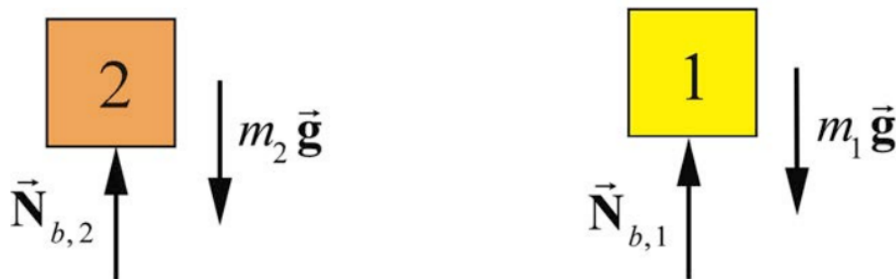
Figure 18.3 Free-body force diagrams for each body.
