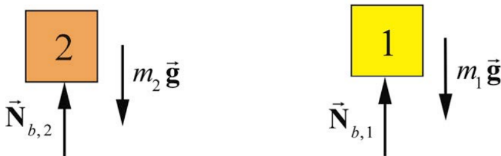
Figure 18.3 Free-body force diagrams for each body.
