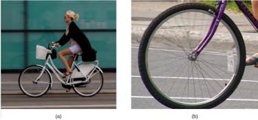
Figure 12.2.1: (a) The bicycle moves forward, and its tires do not slip. The bottom of the slightly deformed tire is at rest with respect to the road surface for a measurable amount of time. (b) This image shows that the top of a rolling wheel appears blurred by its motion, but the bottom of the wheel is instantaneously at rest. (credit a: modification of work by Nelson Lourenço; credit b: modification of work by Colin Rose)
