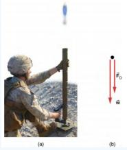
Figure 7.3.8: (a) The mortar fires a shell straight up; we consider the friction force provided by the air. (b) A free-body diagram is shown which indicates all the forces on the mortar shell.
