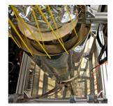
Figure 1.3.2: An atomic clock such as this one uses the vibrations of cesium atoms to keep time to a precision of better than a microsecond per year. The fundamental unit of time, the second, is based on such clocks. This image looks down from the top of an atomic fountain nearly 30 feet tall. (credit: Steve Jurvetson)
