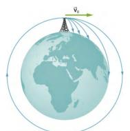
Figure 4.4.7: Projectile to satellite. In each case shown here, a projectile is launched from a very high tower to avoid air resistance. With increasing initial speed, the range increases and becomes longer than it would be on level ground because Earth curves away beneath its path. With a speed of 8000 m/s, orbit is achieved.
