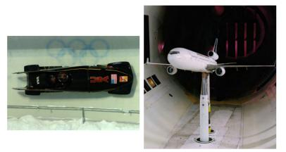
Figure 7.7.1: (A) From racing cars to bobsled racers, aerodynamic shaping is crucial to achieving top speeds. Bobsleds are designed for speed and are shaped like a bullet with tapered fins. (credit: "U.S. Army"/Wikimedia Commons) (B): NASA researchers test a model plane in a wind tunnel. (credit: NASA/Ames).
