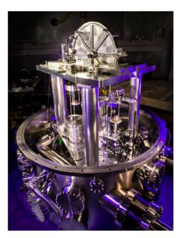
Figure 1.3.4: Redefining the SI unit of mass. The U.S. National Institute of Standards and Technology's Kibble balance is a machine that balances the weight of a test mass with the resulting electrical current needed for a force to balance it.
