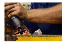
Figure 9.3.1: A grinding wheel applies a non-conservative force, because the work done depends on how many rotations the wheel makes, so it is path-dependent.
