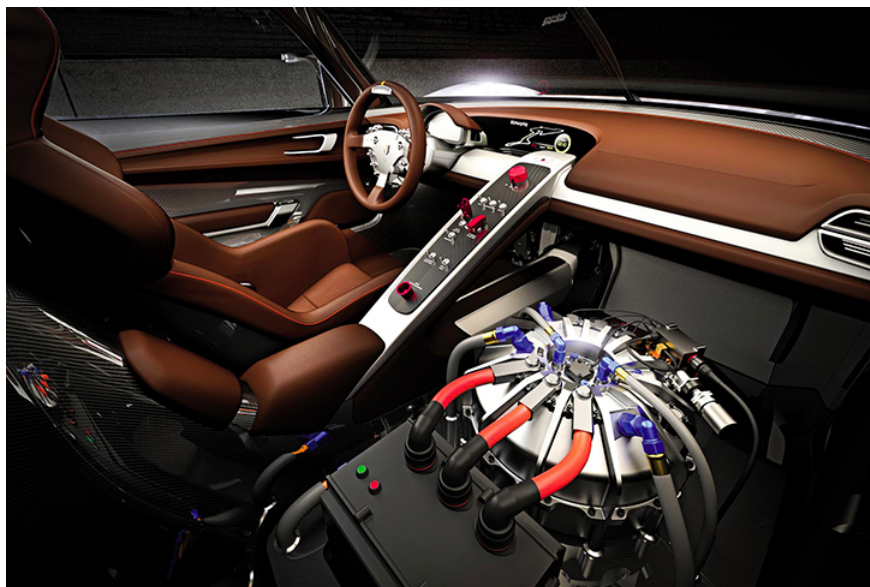
Figure 11.5.2: A KERS (kinetic energy recovery system) flywheel used in cars. (credit: "cmonville"/Flickr)
