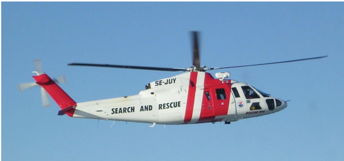
Figure 12.1.1: A helicopter has its main lift blades rotating to keep the aircraft airborne. Due to conservation of angular momentum, the body of the helicopter would want to rotate in the opposite sense to the blades, if it were not for the small rotor on the tail of the aircraft, which provides thrust to stabilize it.
