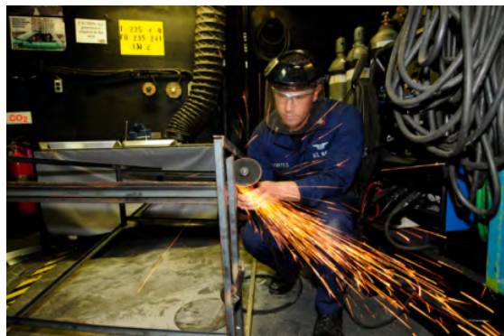
Figure 11.5.1: The rotational kinetic energy of the grindstone is converted to heat, light, sound, and vibration. (credit: Zachary David Bell, US Navy)
