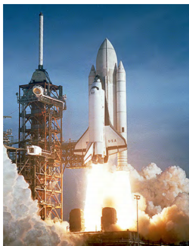
Figure 10.11.1: The space shuttle had a number of reusable parts. Solid fuel boosters on either side were recovered and refueled after each flight, and the entire orbiter returned to Earth for use in subsequent flights. The large liquid fuel tank was expended. The space shuttle was a complex assemblage of technologies, employing both solid and liquid fuel, and pioneering ceramic tiles as reentry heat shields. As a result, it permitted multiple launches as opposed to single-use rockets. (credit: modification of work by NASA)
