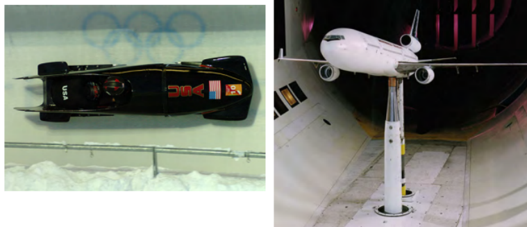
Figure 7.7.1: (A) From racing cars to bobsled racers, aerodynamic shaping is crucial to achieving top speeds. Bobsleds are designed for speed and are shaped like a bullet with tapered fins. (credit: "U.S. Army"/Wikimedia Commons) (B): NASA researchers test a model plane in a wind tunnel. (credit: NASA/Ames).
