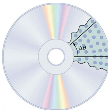
Figure 5.2.1: All points on a CD travel in circular arcs. The pits along a line from the center to the edge all move through the same angle \Delta\theta in a time \Delta t .
