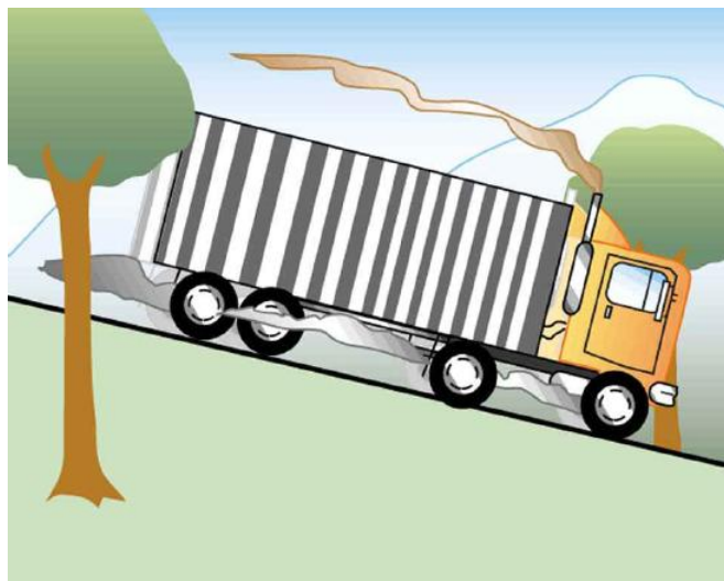
Figure 8.3.2: The smoking brakes on this truck are a visible evidence of the mechanical equivalent of heat.
