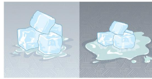
Figure 8.8.3: This illustration shows that the darker pavement is hotter than the lighter pavement (much more of the ice on the right has melted), although both have been in the sunlight for the same time. The thermal conductivities of the pavements are the same.
