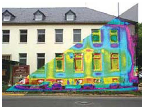
Figure 8.8.5: A thermograph of part of a building shows temperature variations, indicating where heat transfer to the outside is most severe. Windows are a major region of heat transfer to the outside of homes. (credit: U.S. Army)
