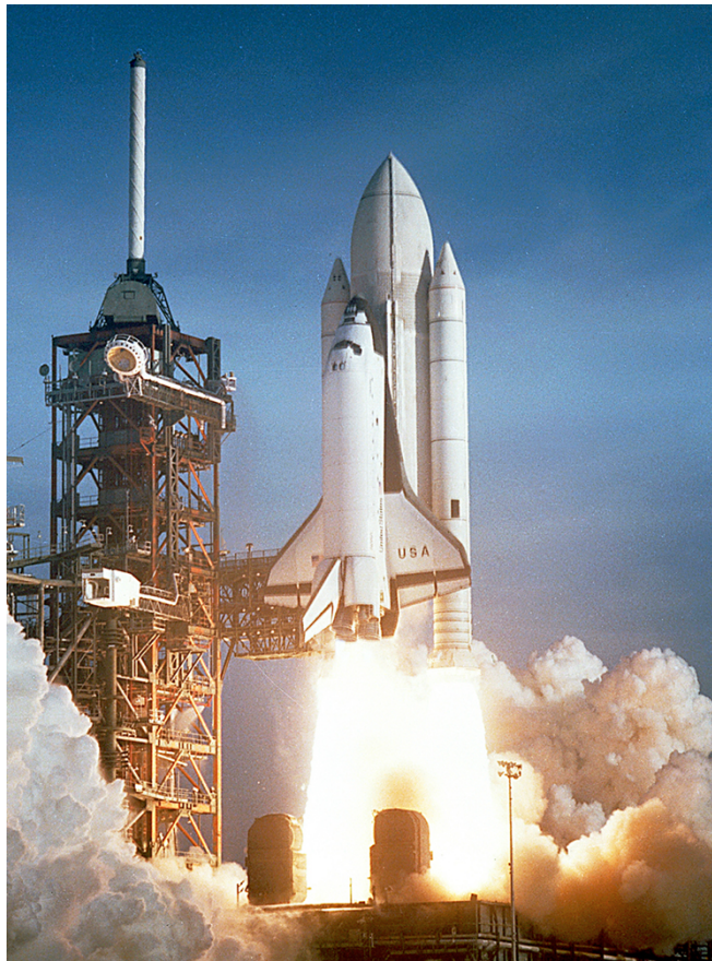
Figure 7.8.2: The space shuttle had a number of reusable parts. Solid fuel boosters on either side were recovered and refueled after each flight, and the entire orbiter returned to Earth for use in subsequent flights. The large liquid fuel tank was expended. The space shuttle was a complex assemblage of technologies, employing both solid and liquid fuel and pioneering ceramic tiles as reentry heat shields. As a result, it permitted multiple launches as opposed to single-use rockets. (credit: NASA)
