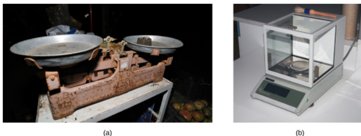
Figure 1.6.1: (a) A double-pan mechanical balance is used to compare different masses. Usually an object with unknown mass is placed in one pan and objects of known mass are placed in the other pan. When the bar that connects the two pans is horizontal, then the masses in both pans are equal. The “known masses” are typically metal cylinders of standard mass such as 1 g, 10 g, and 100 g. (b) Many mechanical balances, such as double-pan balances, have been replaced by digital scales, which can typically measure the mass of an object more precisely. A mechanical balance may read only the mass of an object to the nearest tenth of a gram, but many digital scales can measure the mass of an object up to the nearest thousandth of a gram. (credit a: modification of work by Serge Melki; credit b: modification of work by Karel Jakubec)
