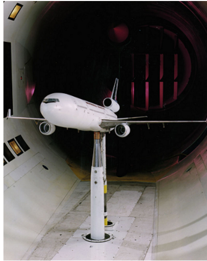
Figure 4.8.2: NASA researchers test a model plane in a wind tunnel. (credit: NASA/Ames)
