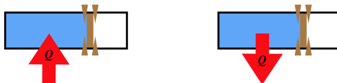
Figure 5.8.1 – Isochoric Processes – Physical Picture
