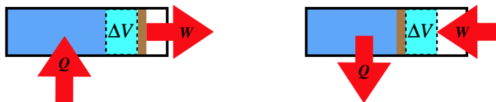
Figure 5.8.3 – Isobaric Processes – Physical Picture
