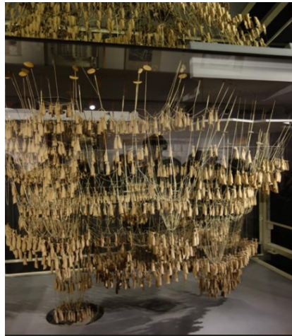
Figure 1.4.4: Gaudi's string model for the Sagrada Família Church
