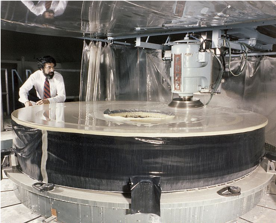
Hubble's primary mirror during fabrication. [ " Hubble mirror polishing " by NASA, in the Public Domain ]
