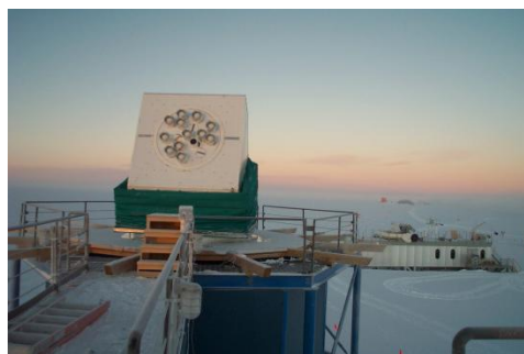
Figure 15.9a: A few of the many instruments used in recent CMB experiments: a close-up of the ACBAR feed horns and electronics, the BOOMERANG telescope , and the WMAP satellite. To date there have been more than 50 experiments designed to measure the CMB. Credits: Acbar Collaboration, NASA/COBE Team, BOOMERANG Collaboration
