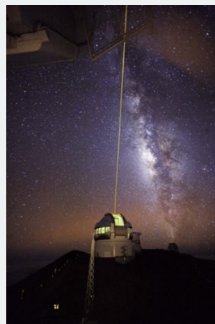
Figure B.7 In this image, the Gemini North telescope on Mauna Kea, Hawaii, is seen against a backdrop of the Milky Way. The observatory sometimes uses a laser beam as part of its adaptive optics system, allowing it to correct for atmospheric distortions and obtain much sharper images than would otherwise be possible. The images can even rival those from the Hubble Space Telescope for sharpness. Gemini North has a twin 8-m telescope, Gemini South, located in the Chilean Andes. Credit: Gemini Observatory/AURA.
