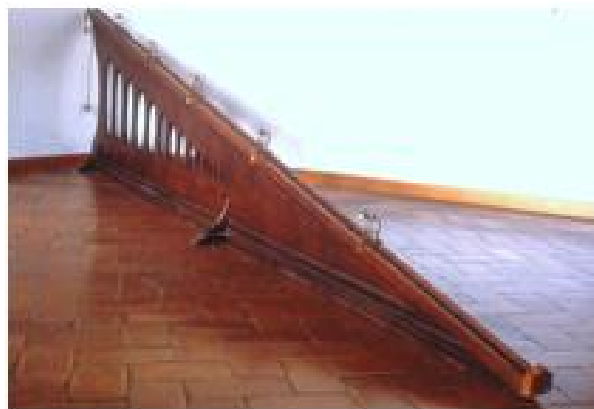
Figure 7.1: Galileo's Experimental Apparatus. Galileo used experiments based upon systems similar to this one to study the motion of falling objects. He also studied the motions of pendula, finding that their periods depend only upon their length, not upon the mass of the object suspended. Credit: Museo Galileo, Florence - Photo Franca Principe
