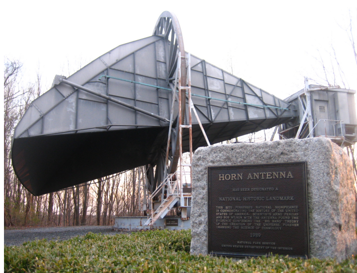
Figure 15.1: This horn antenna was used by Penzias and Wilson at Bell Labs in their discovery of the CMB. Credit: Wikimedia Commons
