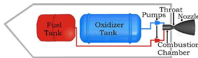
Schematic of the liquid fuel rocket. https://commons.wikimedia.org/wiki/File:LiquidFuelRocketSchematic.jpg ;
