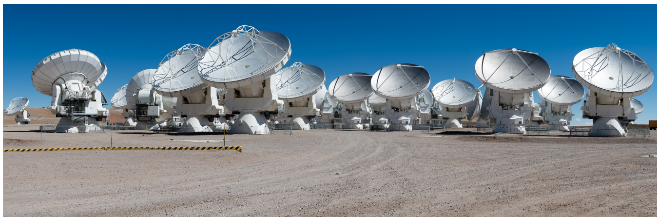
ALMA: The Atacama Large Millimeter/Submillimeter Array uses multiple radio dishes to improve resolution through interferometry.
