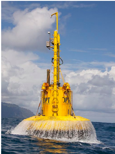
Figure 12.1.1: From the world of renewable energy sources comes the electric power-generating buoy. Although there are many versions, this one converts the up-and-down motion, as well as side-to-side motion, of the buoy into rotational motion in order to turn an electric generator, which stores the energy in batteries.
