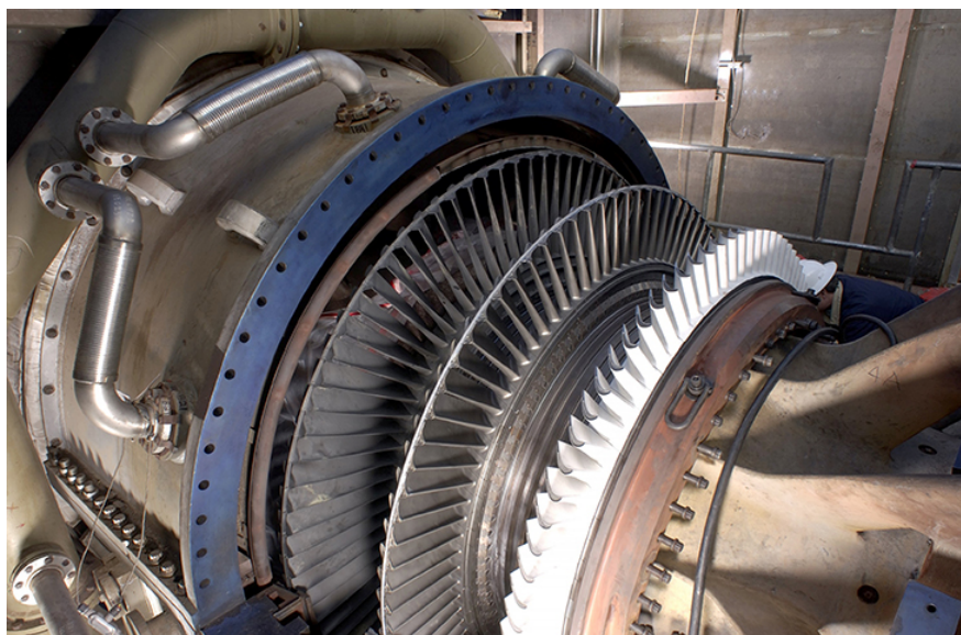
Figure 9.7.5: Steam turbine/generator. The steam produced by burning coal impacts the turbine blades, turning the shaft, which is connected to the generator.
