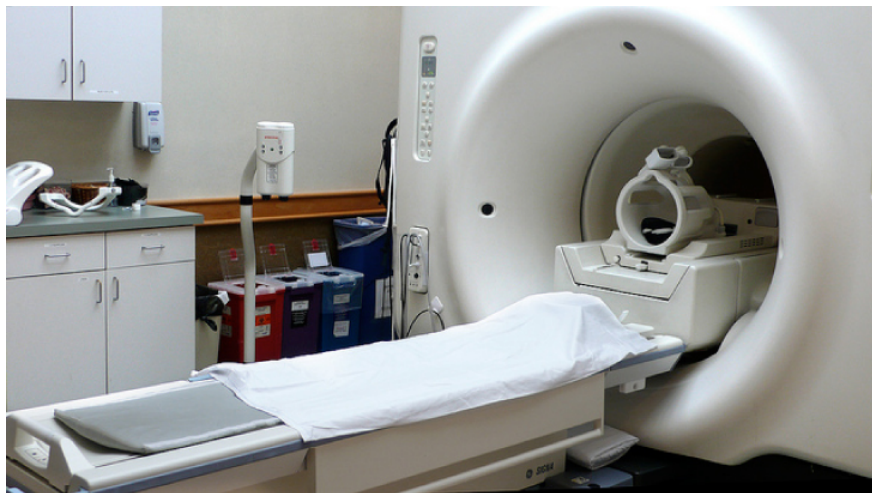
Figure 8.7.3: . In an MRI machine, a large magnetic field is generated by the cylindrical solenoid surrounding the patient. (credit: Liz West)
