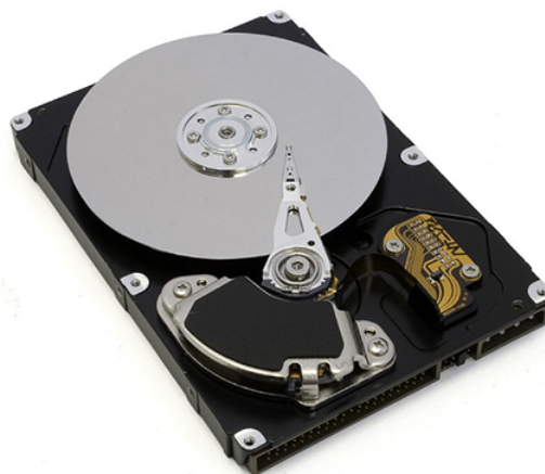
Figure 8.8.6: The inside of a hard disk drive. The silver disk contains the information, whereas the thin stylus on top of the disk reads and writes information to the disk.
