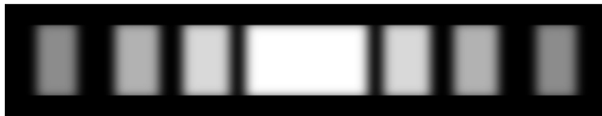
Figure 14.3.3: (a) The calculated intensity distribution of a single-slit diffraction pattern. (b) The actual diffraction pattern.
