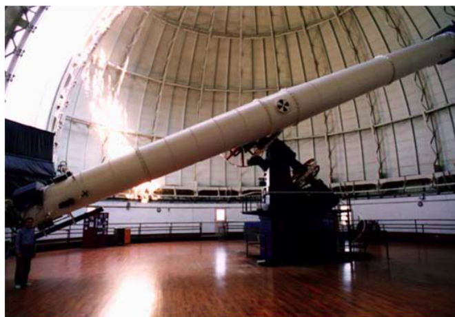
Figure 11.9.6: In 1897, the Yerkes Observatory in Wisconsin (USA) built a large refracting telescope with an objective lens that is 40 inches in diameter and has a tube length of 62 feet. (credit: Yerkes Observatory, University of Chicago)
