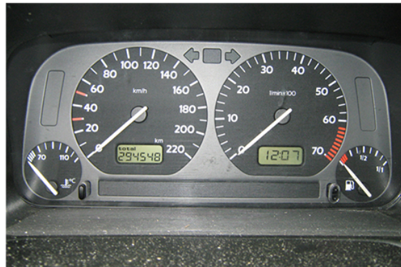
Figure 6.5.1: The fuel and temperature gauges (far right and far left, respectively) in this 1996 Volkswagen are voltmeters that register the voltage output of “sender” units. These units are proportional to the amount of gasoline in the tank and to the engine temperature. (credit: Christian Giersing)
