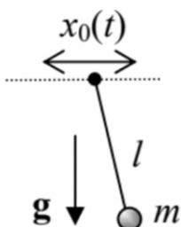
2.4. A pendulum of mass  $m$ , hung on another point mass  $m'$ , which may slide, without friction, along a straight horizontal rail - see the figure on the right. The motion is confined to the vertical plane that contains the rail.
