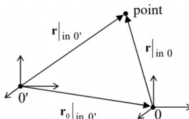
Figure 1.2. Transfer between two reference frames.
