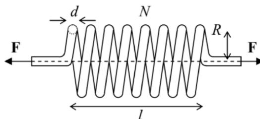
7.13. The coil spring, described in the previous problem, is now used as what is sometimes called the torsion spring - see the figure on the right. Find the corresponding spring constant  $d\tau/d\varphi$ , where  $\tau$  is the torque of the external forces relative to the center of the coil (point 0).
