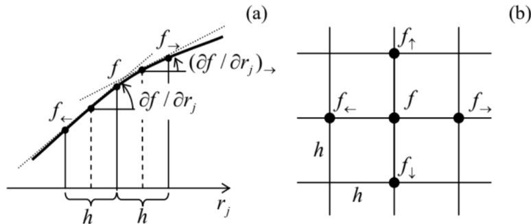
Figure 8.13. The idea of the finite-difference method in (a) one and (b) two dimensions.
