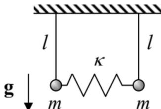
6.2. The double pendulum, confined to a vertical plane containing the support point (considered in Problem 2.1), with  $m' = m$  and  $l = l'$  – see the figure on the right.
