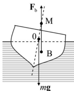
Figure 8.3. Angular stability of a floating body.
