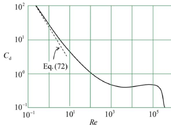
Figure 8.15. The drag coefficient  $C_d$  for a sphere in an incompressible fluid, as a function of the Reynolds number (Note the log – log plot). The experimental data are from F. Eisner, *Das Widerstandsproblem*, in: Proc. 3<sup>rd</sup> Int. Congress on Appl. Mech., Stockholm, 1931.
