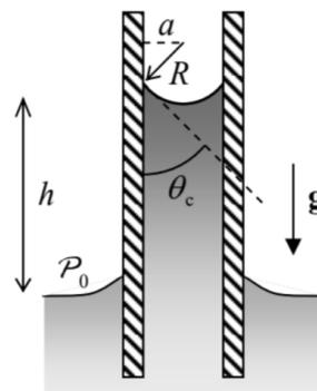
Figure 8.6. Liquid's rise in a vertical capillary tube.
