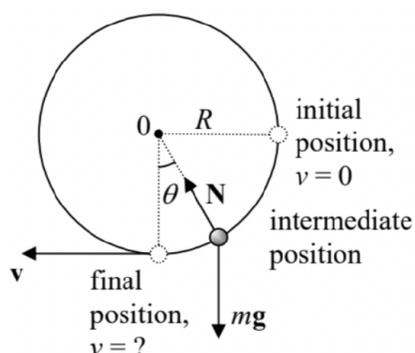
Figure 1.3. A bead sliding along a vertical ring.
