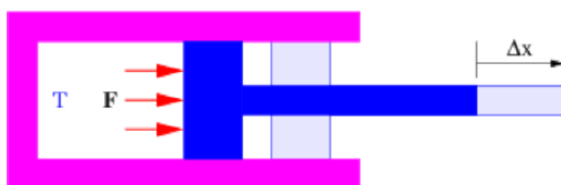
Figure 22.2.2:: Conversion of internal energy of gas in the cylinder to macroscopic energy. The work done by the force of the gas on the piston as it moves outward results in a decrease in temperature of the gas.
