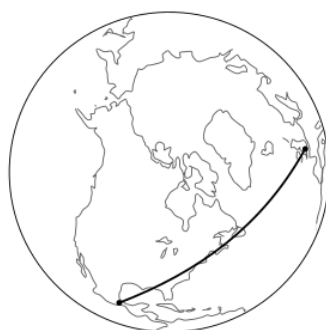
Figure 2.2.1: An airplane flying from Mexico City to London follows the shortest path, which is a segment of a great circle. A path of extremal length between two points is called a geodesic.
