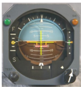
Figure 5.2.2: An artificial horizon.
