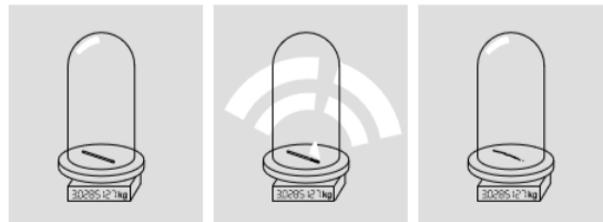
Figure 4.2.1: The match is lit inside the bell jar. It burns, and energy escapes from the jar in the form of light. After it stops burning, all the same atoms are still in the jar: none have entered or escaped. The figure shows the outcome expected before relativity, which was that the mass measured on the balance would remain exactly the same. This is not what happens in reality.
