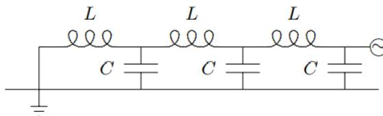
Figure 5.29: A forced oscillation with three inductors.
