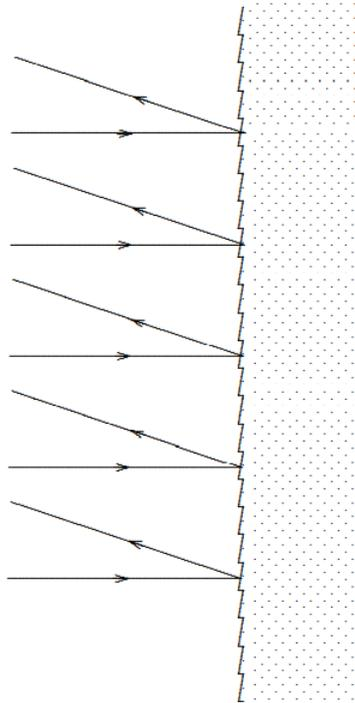
Figure 13.24: The grooves of a blazed grating.
