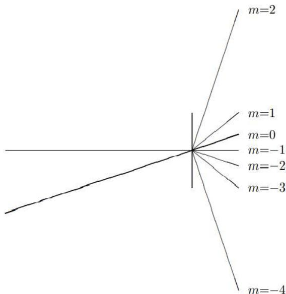
Figure 13.19: The pattern for a beam at an angle,  $\theta_{\text{in}} = \arcsin \lambda/a$ .
