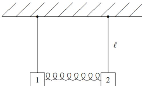
Figure 3.1: Two pendulums coupled by a spring.
