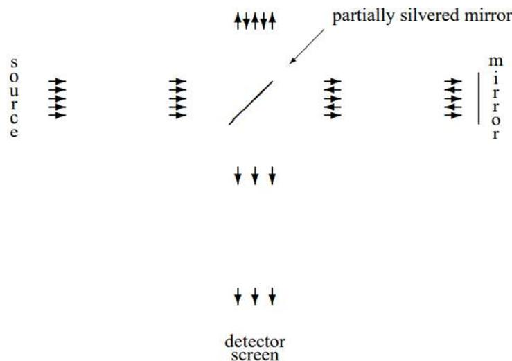
Figure 8.8: A schematic diagram of a Michelson interferometer.
