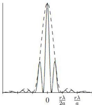
Figure 13.16: The diffraction pattern for two wide slits.
