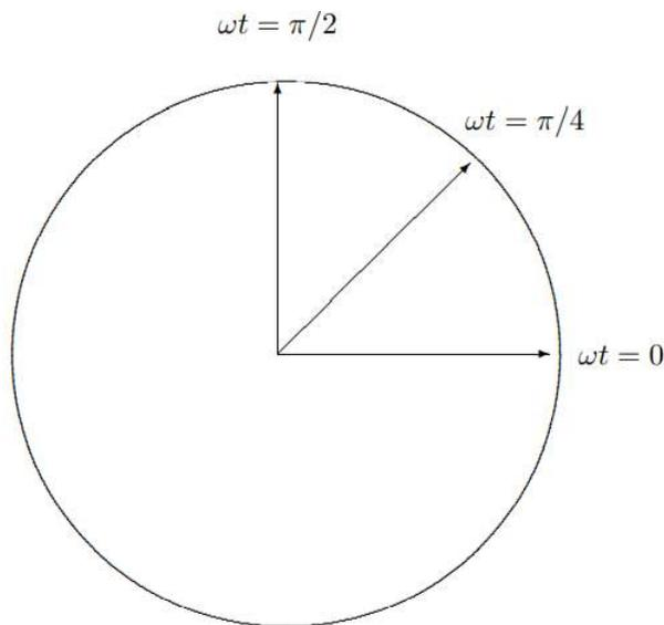
Figure 12.2: Circular polarization.
