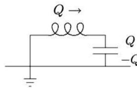
Figure 1.12: The charge moved through the inductor.
