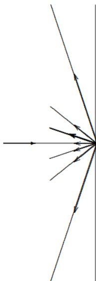
Figure 13.23: A blazed grating directs the beam into a nontrivial diffraction maximum.
