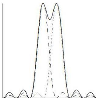
Figure 13.21: Rayleigh's criterion for a grating with 6 lines.
