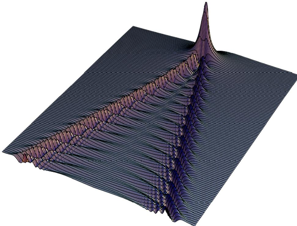
Figure 14.3: A wake constructed numerically from (14.3) for  $f(\omega) = e^{-\omega^2 v/g}$ .
