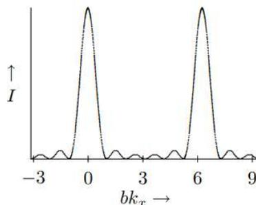
Figure 13.14: The diffraction pattern for 6 narrow slits.
