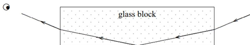
Figure 11.10: Total internal reflection in glass with index of refraction 2.
