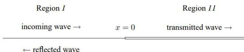
Figure 9.1: Two semi-infinite strings tied together at  $x = 0$ .
