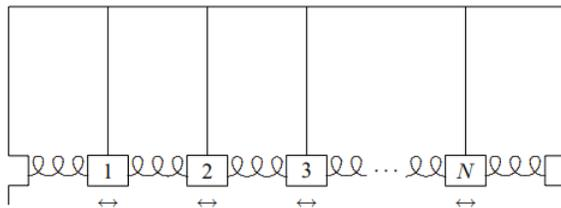
Figure 5.1: A finite system of coupled pendulums.
