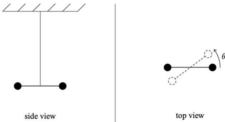
Figure 1.14: Two views of a torsion pendulum.
