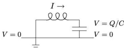
Figure 1.13: Voltage and current.
