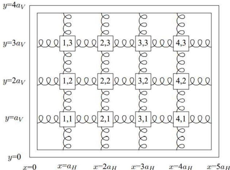
Figure 11.4: A two-dimensional system of beads and springs.
