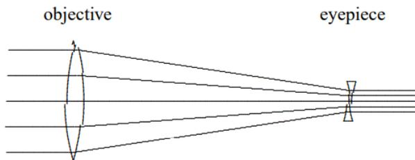
The focal length of the convex lens is  $f_1$  and the focal length of the concave lens is  $-f_2$ .
