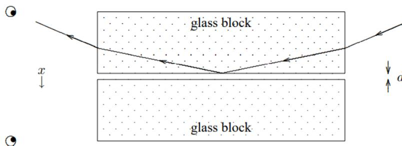
Figure 11.11: A simple experiment to demonstrate tunneling.
