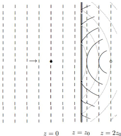
Figure 13.36: A plane wave illuminating the photographic plate.
