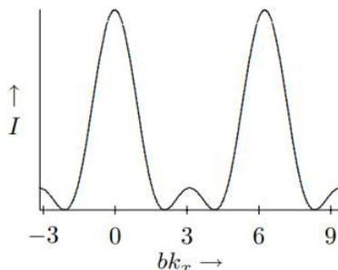
Figure 13.13: The diffraction pattern for three narrow slits.
