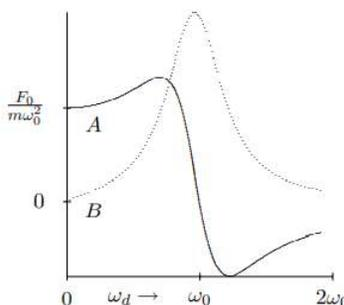
Figure 2.4: The elastic and absorptive amplitudes, plotted versus  $\omega_d$ . The absorptive amplitude is the dotted line.
