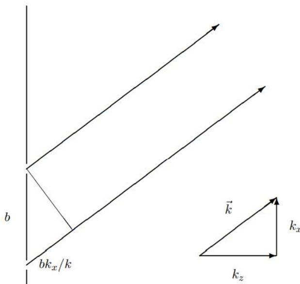
Figure 13.12: If  $bk_x/k = n\lambda$ , the interference is constructive.
