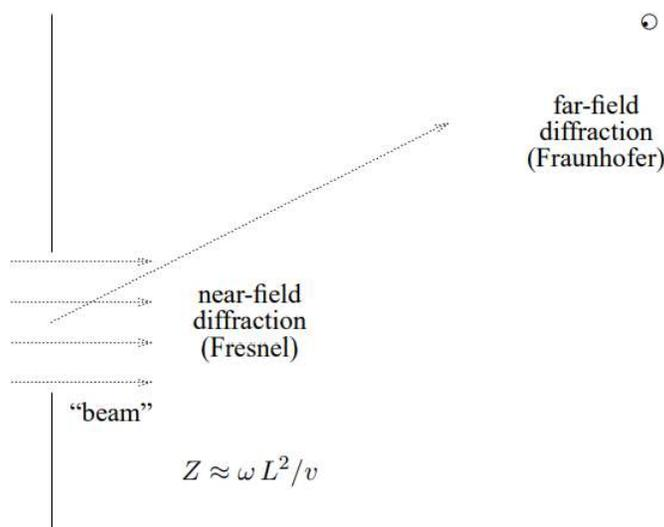
Figure 13.3: The basic diffraction problem — making a beam.
