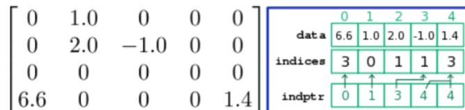
Figure 8.2.4: A sparse matrix and its representation in Compressed Sparse Column (CSC) format.
