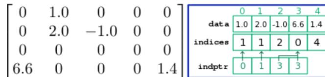
Figure 8.2.3: A sparse matrix and its representation in Compressed Sparse Row (CSR) format.
