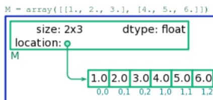
Figure 4.1.1: Memory model of a 2D array.
