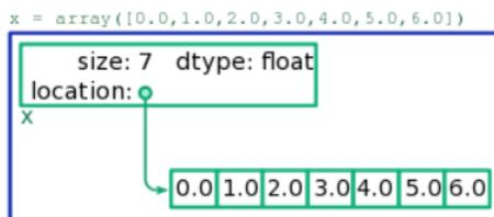
Figure 3.3.1: Schematic of how an array is laid out in memory. The book-keeping block (upper left box) records the array size, the address of the storage blocks (indicated by an arrow), etc. The storage blocks (lower right boxes) contain the array contents, in sequential order.
