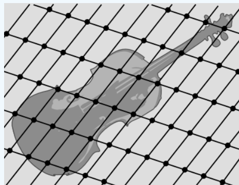
Figure 2.2.6 - The area of the viola can be determined by counting the parallelograms formed by the lattice. The area can be determined to any desired precision, by dividing the parallelograms into fractional parts that are as small as necessary.
