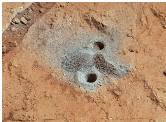
Figure 30.3.1 Mudstone. Shown are the first holes drilled by NASA's Curiosity Mars rover into a mudstone, with “fresh” drill-pilings around the holes. Notice the difference in color between the red ancient martian surface and the gray newly exposed rock powder that came from the drill holes. Each drill hole is about 0.6 inch (1.6 cm) in diameter.
