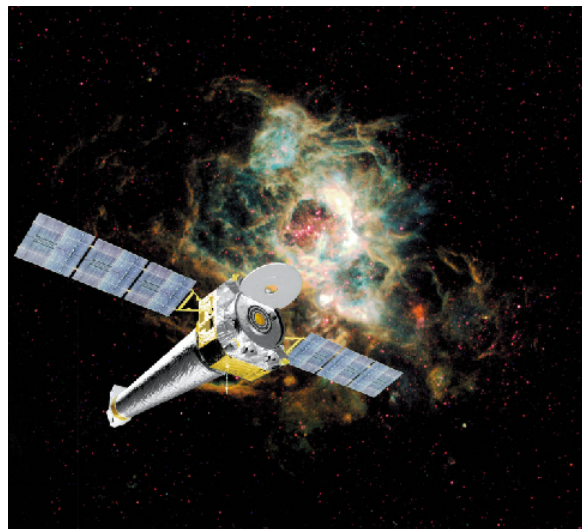
Figure 6.5.4 Chandra X-Ray Satellite. Chandra, the world's most powerful X-ray telescope, was developed by NASA and launched in July 1999.
