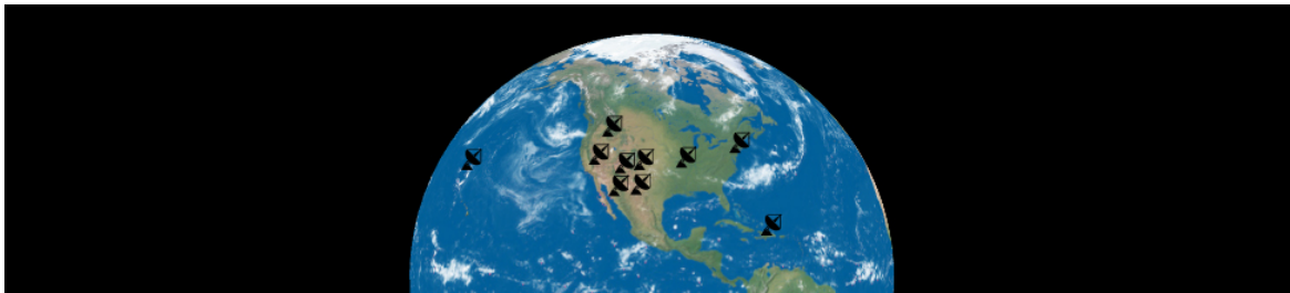
Figure 6.4.5 Very Long Baseline Array. This map shows the distribution of 10 antennas that constitute an array of radio telescopes stretching across the United States and its territories.
