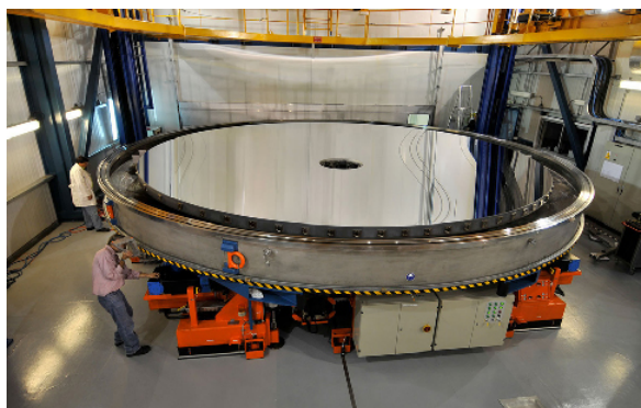
Figure 6.2.1 Large Telescope Mirror. This image shows one of the primary mirrors of the European Southern Observatory's Very Large Telescope, named Yepun, just after it was recoated with aluminum. The mirror is a little over 8 meters in diameter.
