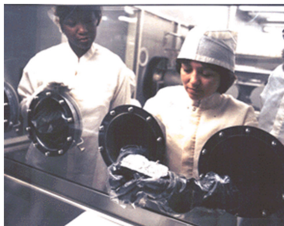
Figure 9.1.3 Handling Moon Rocks. Lunar samples collected in the Apollo Project are analyzed and stored in NASA facilities at the Johnson Space Center in Houston, Texas. Here, a technician examines a rock sample using gloves in a sealed environment to avoid contaminating the sample.
