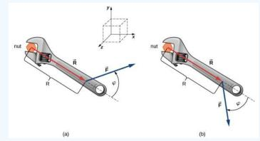
Figure 2.9.3: A wrench provides grip and mechanical advantage in applying torque to turn a nut. (a) Turn counterclockwise to loosen the nut. (b) Turn clockwise to tighten the nut.
