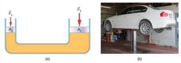
Figure 14.5.3: (a) A hydraulic jack operates by applying forces  $(F_1, F_2)$  to an incompressible fluid in a U-tube, using a movable piston  $(A_1, A_2)$  on each side of the tube. (b) Hydraulic jacks are commonly used by car mechanics to lift vehicles so that repairs and maintenance can be performed.
