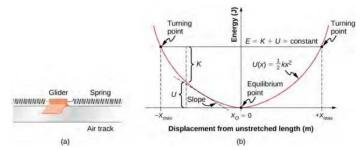
Figure 8.5.2: (a) A glider between springs on an air track is an example of a horizontal mass-spring system. (b) The potential energy diagram for this system, with various quantities indicated.
