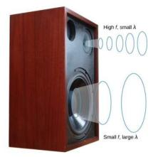
Figure 17.3.7: Because they travel at the same speed in a given medium, low-frequency sounds must have a greater wavelength than high-frequency sounds. Here, the lower-frequency sounds are emitted by the large speaker, called a woofer, whereas the higher-frequency sounds are emitted by the small speaker, called a tweeter.
