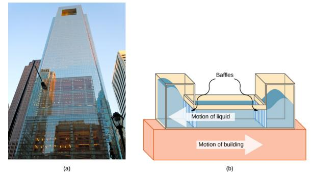
Figure 15.1.1: (a) The Comcast Building in Philadelphia, Pennsylvania, looming high above the skyline, is approximately 305 meters (1000 feet) tall. At this height, the top floors can oscillate back and forth due to seismic activity and fluctuating winds. (b) Shown above is a schematic drawing of a tuned, liquid-column mass damper, installed at the top of the Comcast, consisting of a 300,000-gallon reservoir of water to reduce oscillations.
