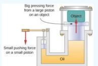
Figure 12.5.2: In a hydraulic press, when a small piston is displaced downward, the pressure in the oil is transmitted throughout the oil to the large piston, causing the large piston to move upward. A small force applied to a small piston causes a large pressing force, which the large piston exerts on an object that is either lifted or squeezed. The device acts as a mechanical lever.
