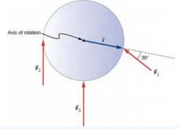
Figure 10.7.5: Three forces acting on a flywheel.
