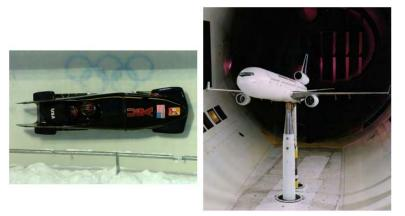
Figure 6.7.1: (A) From racing cars to bobsled racers, aerodynamic shaping is crucial to achieving top speeds. Bobsleds are designed for speed and are shaped like a bullet with tapered fins. (credit: "U.S. Army"/Wikimedia Commons) (B): NASA researchers test a model plane in a wind tunnel. (credit: NASA/Ames).
