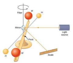
Figure 13.2.1: Cavendish used an apparatus similar to this to measure the gravitational attraction between two spheres (m) suspended from a wire and two stationary spheres (M). This is a common experiment performed in undergraduate laboratories, but it is quite challenging. Passing trucks outside the laboratory can create vibrations that overwhelm the gravitational forces.
