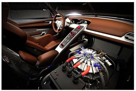
Figure 10.5.2: A KERS (kinetic energy recovery system) flywheel used in cars. (credit: "cmonville"/Flickr)
