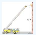
Figure 14.8.5: Pressure in the nozzle of this fire hose is less than at ground level for two reasons: The water has to go uphill to get to the nozzle, and speed increases in the nozzle. In spite of its lowered pressure, the water can exert a large force on anything it strikes by virtue of its kinetic energy. Pressure in the water stream becomes equal to atmospheric pressure once it emerges into the air.
