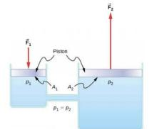
Figure 14.5.2: A typical hydraulic system with two fluid-filled cylinders, capped with pistons and connected by a tube called a hydraulic line. A downward force  $\vec{F}_1$  on the left piston creates a change in pressure that is transmitted undiminished to all parts of the enclosed fluid. This results in an upward force  $\vec{F}_2$  on the right piston that is larger than  $\vec{F}_1$  because the right piston has a larger surface area.
