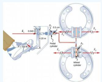
Figure 14.5.4: Hydraulic brakes use Pascal's principle. The driver pushes the brake pedal, exerting a force that is increased by the simple lever and again by the hydraulic system. Each of the identical wheel cylinders receives the same pressure and, therefore, creates the same force output  $F_2$ . The circular cross-sectional areas of the pedal and wheel cylinders are represented by  $A_1$  and  $A_2$ , respectively
