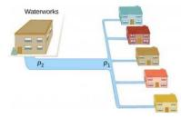
Figure 14.9.6: During times of heavy use, there is a significant pressure drop in a water main, and  $p_1$  supplied to users is significantly less than  $p_2$  created at the water works. If the flow is very small, then the pressure drop is negligible, and  $p_2 \approx p_1$ .
