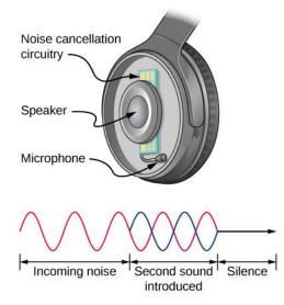
Figure 17.5.3: Headphones designed to cancel noise with destructive interference create a sound wave exactly opposite to the incoming sound. These headphones can be more effective than the simple passive attenuation used in most ear protection. Such headphones were used on the record-setting, around-the-world nonstop flight of the *Voyager* aircraft in 1986 to protect the pilots' hearing from engine noise.
