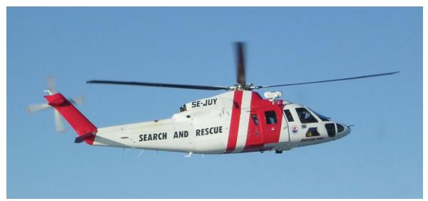
Figure 11.1.1: A helicopter has its main lift blades rotating to keep the aircraft airborne. Due to conservation of angular momentum, the body of the helicopter would want to rotate in the opposite sense to the blades, if it were not for the small rotor on the tail of the aircraft, which provides thrust to stabilize it.
