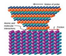
Figure 6.5.3: The tip of a probe is deformed sideways by frictional force as the probe is dragged across a surface. Measurements of how the force varies for different materials are yielding fundamental insights into the atomic nature of friction.
