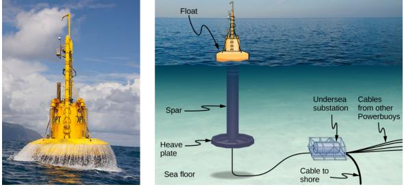
Figure 16.1.1: From the world of renewable energy sources comes the electric power-generating buoy. Although there are many versions, this one converts the up-and-down motion, as well as side-to-side motion, of the buoy into rotational motion in order to turn an electric generator, which stores the energy in batteries.
