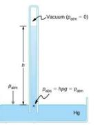
Figure 14.4.3: A mercury barometer measures atmospheric pressure. The pressure due to the mercury's weight,  $h\rho g$ , equals atmospheric pressure. The atmosphere is able to force mercury in the tube to a height h because the pressure above the mercury is zero.
