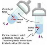
Figure 6.6.7: Centrifuges use inertia to perform their task. Particles in the fluid sediment settle out because their inertia carries them away from the center of rotation. The large angular velocity of the centrifuge quickens the sedimentation. Ultimately, the particles come into contact with the test tube walls, which then supply the centripetal force needed to make them move in a circle of constant radius.
