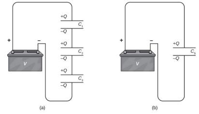
Figure 8.3.1: (a) Three capacitors are connected in series. The magnitude of the charge on each plate is Q. (b) The network of capacitors in (a) is equivalent to one capacitor that has a smaller capacitance than any of the individual capacitances in (a), and the charge on its plates is Q.
