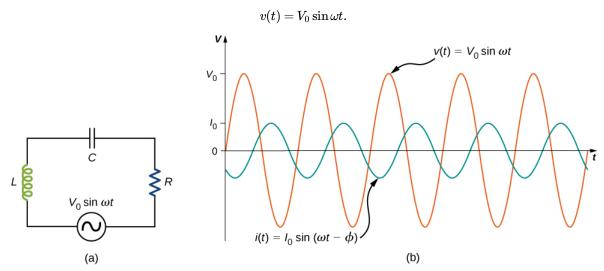
Figure 15.4.1: (a) An RLC series circuit. (b) A comparison of the generator output voltage and the current. The value of the phase difference  $\phi$  depends on the values of R, C, and L.
