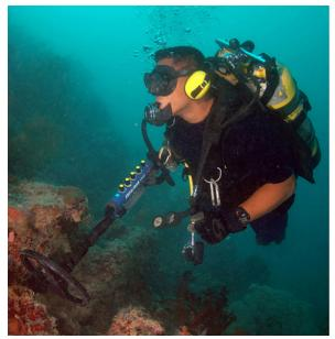
Figure 15.6.3: When a metal detector comes near a piece of metal, the self-inductance of one of its coils changes. This causes a shift in the resonant frequency of a circuit containing the coil. That shift is detected by the circuitry and transmitted to the diver by means of the headphones.
