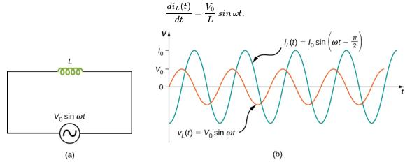
Figure 15.3.6: (a) An inductor connected across an ac generator. (b) The current  $i_L(t)$  through the inductor and the voltage  $v_L(t)$  across the inductor. Here  $i_L(t)$  lags  $v_L(t)$  by  $\pi/2$  rad.
