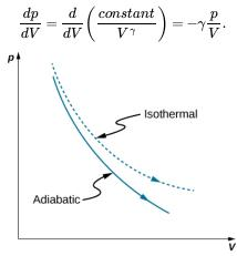
Figure 3.7.3: Quasi-static adiabatic and isothermal expansions of an ideal gas.
