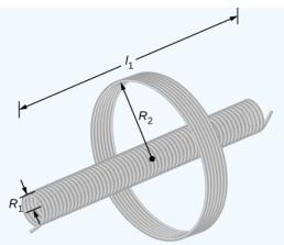
Figure 14.2.3: A solenoid surrounded by a coil.
