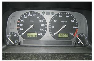
Figure 10.5.1: The fuel and temperature gauges (far right and far left, respectively) in this 1996 Volkswagen are voltmeters that register the voltage output of "sender" units. These units are proportional to the amount of gasoline in the tank and to the engine temperature. (credit: Christian Giersing)
