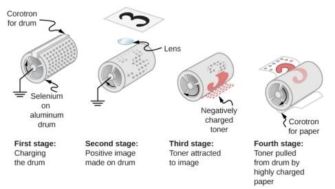
Figure 7.7.2: Xerography is a dry copying process based on electrostatics. The major steps in the process are the charging of the photoconducting drum, transfer of an image, creating a positive charge duplicate, attraction of toner to the charged parts of the drum, and transfer of toner to the paper. Not shown are heat treatment of the paper and cleansing of the drum for the next copy.
