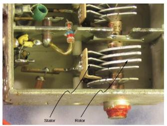
Figure 8.2.7: In a variable air capacitor, capacitance can be tuned by changing the effective area of the plates. (credit: modification of work by Robbie Sproule)
