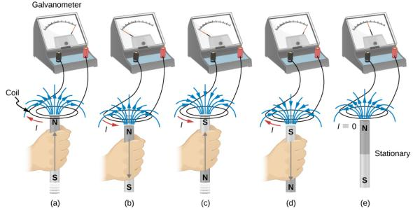
Figure 13.2.1: Movement of a magnet relative to a coil produces emfs as shown (a–d). The same emfs are produced if the coil is moved relative to the magnet. This short-lived emf is only present during the motion. The greater the speed, the greater the magnitude of the emf, and the emf is zero when there is no motion, as shown in (e).
