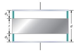
**82.** A parallel-plate capacitor is filled with two dielectrics, as shown below. When the plate area is A and separation between plates is d, show that the capacitance is given by  $C = \varepsilon_0 \frac{A}{d} \frac{\kappa_1 + \kappa_2}{2}$ .
