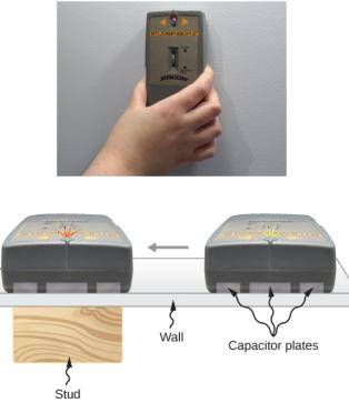
Figure 8.5.2: An electronic stud finder is used to detect wooden studs behind drywall.
