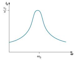
Figure 15.6.1: At an RLC circuit's resonant frequency,  $\omega_0 = \sqrt{1/LC}$ , the current amplitude is at its maximum value.
