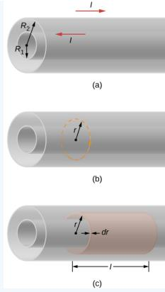
Figure 14.4.1: (a) A coaxial cable is represented here by two hollow, concentric cylindrical conductors along which electric current flows in opposite directions. (b) The magnetic field between the conductors can be found by applying Ampère's law to the dashed path. (c) The cylindrical shell is used to find the magnetic energy stored in a length **l** of the cable.
