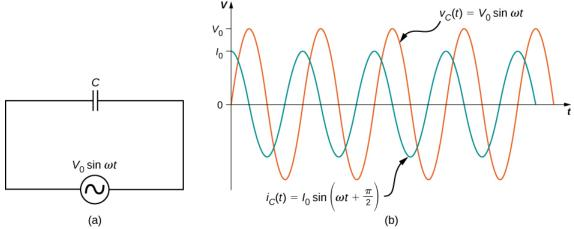
Figure 15.3.4: (a) A capacitor connected across an ac generator. (b) The current  $i_C(t)$  through the capacitor and the voltage  $v_C(t)$  across the capacitor. Notice that  $i_C(t)$  leads  $v_C(t)$  by  $\pi/2$  rad.
