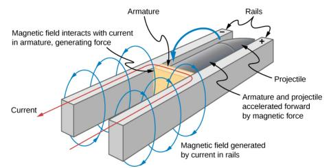
Figure 13.4.3: Current through two rails drives a conductive projectile forward by the magnetic force created.
