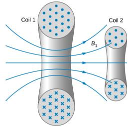
Figure 14.2.1: Some of the magnetic field lines produced by the current in coil 1 pass through coil 2.
