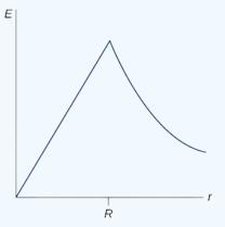
Figure 13.5.2: The electric field vs. distance **r**. When r < R, the electric field rises linearly, whereas when r > R, the electric field falls of proportional to 1/r.
