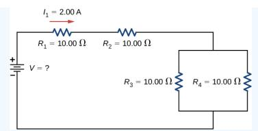
Figure 10.3.8: To find the unknown voltage, we must first find the equivalent resistance of the circuit.
