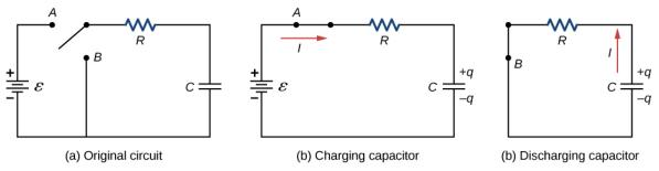
Figure 10.6.1: (a) An **RC** circuit with a two-pole switch that can be used to charge and discharge a capacitor. (b) When the switch is moved to position **A**, the circuit reduces to a simple series connection of the voltage source, the resistor, the capacitor, and the switch. (c) When the switch is moved to position **B**, the circuit reduces to a simple series connection of the resistor, the capacitor, and the switch. The voltage source is removed from the circuit.
