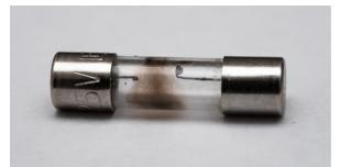
Figure 9.6.3: A fuse consists of a piece of wire between two contacts. When a current passes through the wire that is greater than the rated current, the wire melts, breaking the connection. Pictured is a "blown" fuse where the wire broke protecting a circuit (credit: modification of work by "Shardayyy"/Flickr).
