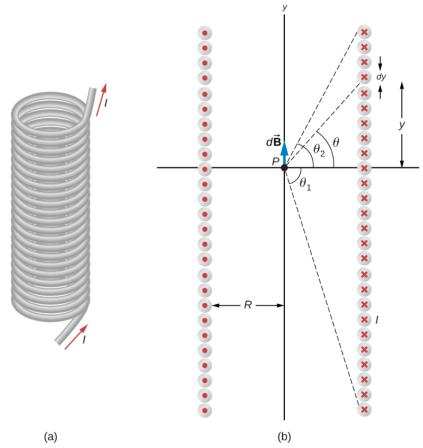
Figure 12.7.1: (a) A solenoid is a long wire wound in the shape of a helix. (b) The magnetic field at the point **P** on the axis of the solenoid is the net field due to all of the current loops.
