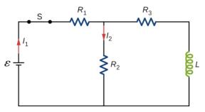
**60.** For the circuit shown below, find the current through the inductor  $2.0 \times 10^{-5} s$  after the switch is reopened.
