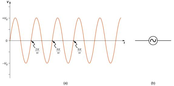
Figure 15.3.1: (a) The output  $v(t) = V_0 \sin \omega t$  of an ac generator. (b) Symbol used to represent an ac voltage source in a circuit diagram.
