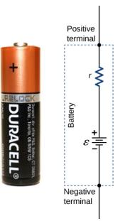
Figure 10.2.5: A battery can be modeled as an idealized emf ( $\epsilon$ ) with an internal resistance (**r**). The terminal voltage of the battery is  $V_{terminal} = \epsilon - Ir$ .
