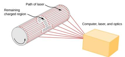
Figure 7.7.3: In a laser printer, a laser beam is scanned across a photoconducting drum, leaving a positively charged image. The other steps for charging the drum and transferring the image to paper are the same as in xerography. Laser light can be very precisely controlled, enabling laser printers to produce high-quality images.
