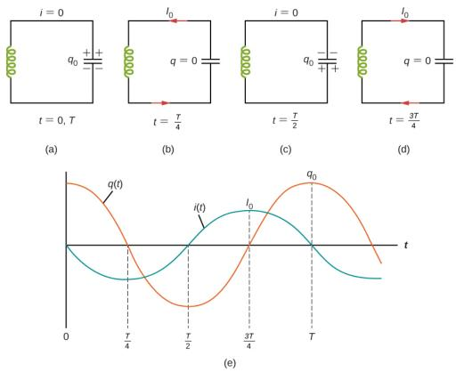
Figure 14.6.1: (a–d) The oscillation of charge storage with changing directions of current in an **LC** circuit. (e) The graphs show the distribution of charge and current between the capacitor and inductor.
