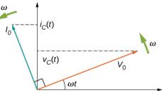
Figure 15.3.5: The current phasor leads the voltage phasor by  $\pi/2$  rad as they both rotate with the same angular frequency.
