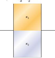
**83.** A parallel-plate capacitor is filled with two dielectrics, as shown below. Show that the capacitance is given by  $C = 2\varepsilon_0 \frac{A}{d} \frac{\kappa_1 \kappa_2}{\kappa_1 + \kappa_2}$ .
