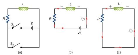
Figure 14.5.1: (a) An RL circuit with switches  $S_1$  and  $S_2$ . (b) The equivalent circuit with  $S_1$  closed and  $S_2$  open. (c) The equivalent circuit after  $S_1$  is opened and  $S_2$  is closed.
