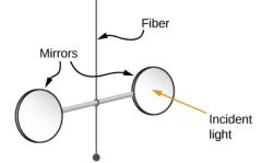
Figure 16.5.2: Simplified diagram of the central part of the apparatus Nichols and Hull used to precisely measure radiation pressure and confirm Maxwell's prediction.
