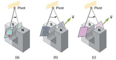
Figure 13.6.1: A common physics demonstration device for exploring eddy currents and magnetic damping. (a) The motion of a metal pendulum bob swinging between the poles of a magnet is quickly damped by the action of eddy currents. (b) There is little effect on the motion of a slotted metal bob, implying that eddy currents are made less effective. (c) There is also no magnetic damping on a nonconducting bob, since the eddy currents are extremely small.
