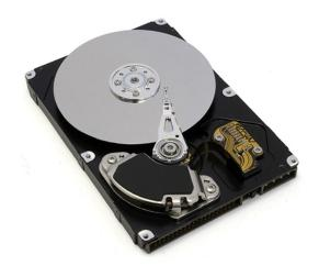
Figure 12.8.6: The inside of a hard disk drive. The silver disk contains the information, whereas the thin stylus on top of the disk reads and writes information to the disk.
