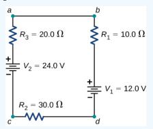
Figure 10.4.12: This circuit consists of three resistors and two batteries connected in series. Note that the batteries are connected with opposite polarities.
