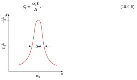
Figure 15.6.2: Like the current, the average power transferred from an ac generator to an **RLC** circuit peaks at the resonant frequency.
