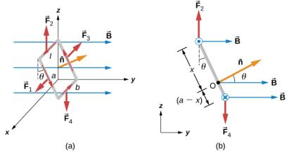
Figure 11.6.2: (a) A rectangular current loop in a uniform magnetic field is subjected to a net torque but not a net force. (b) A side view of the coil.
