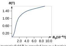
Figure 12.8.3: (a) The magnetic field B in annealed iron as a function of the applied field  $B_0$ .
