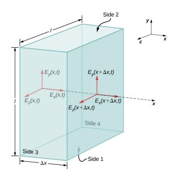
Figure 16.3.1: The surface of a rectangular box of dimensions  $l \times l \times \Delta x$  is our Gaussian surface. The electric field shown is from an electromagnetic wave propagating along the x-axis.
