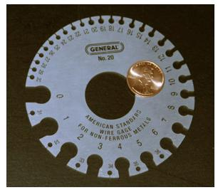
Figure 9.3.5: A device for measuring the gauge of electrical wire. As you can see, higher gauge numbers indicate thinner wires.
