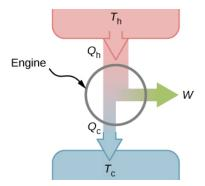
Figure 4.3.1: A schematic representation of a heat engine. Energy flows from the hot reservoir to the cold reservoir while doing work.
