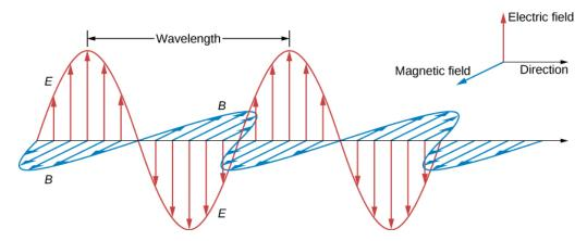
Figure 16.3.3: The plane wave solution of Maxwell's equations has the B field directly proportional to the E field at each point, with the relative directions shown.
