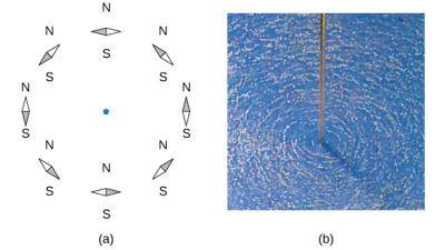
Figure 12.3.3: The shape of the magnetic field lines of a long wire can be seen using (a) small compass needles and (b) iron filings.
