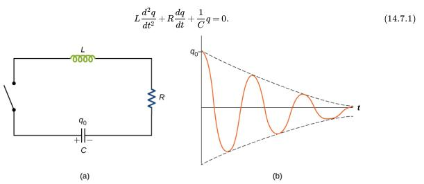
Figure 14.7.1: (a) An **RLC** circuit. Electromagnetic oscillations begin when the switch is closed. The capacitor is fully charged initially. (b) Damped oscillations of the capacitor charge are shown in this curve of charge versus time, or **q** versus **t**. The capacitor contains a charge  $q_0$  before the switch is closed.
