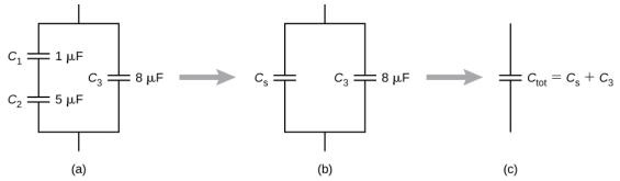
Figure 8.3.3: (a) This circuit contains both series and parallel connections of capacitors. (b)  $C_1$  and  $C_2$  are in series; their equivalent capacitance is  $C_S$  c) The equivalent capacitance  $C_S$  is connected in parallel with  $C_3$ . Thus, the equivalent capacitance of the entire network is the sum of  $C_S$  and  $C_3$ .
