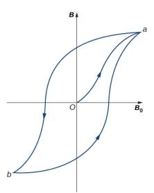
Figure 12.8.4: A typical hysteresis loop for a ferromagnet. When the material is first magnetized, it follows a curve from 0 to **a**. When  $B_0$  is reversed, it takes the path shown from **a** to **b**. If  $B_0$  is reversed again, the material follows the curve from **b** to **a**.
