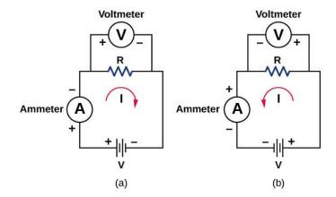
Figure 9.5.1: The experimental set-up used to determine if a resistor is an ohmic or nonohmic device. (a) When the battery is attached, the current flows in the clockwise direction and the voltmeter and ammeter have positive readings. (b) When the leads of the battery are switched, the current flows in the counterclockwise direction and the voltmeter and ammeter have negative readings.
