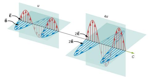
Figure 16.4.1: Energy carried by a wave depends on its amplitude. With electromagnetic waves, doubling the **E** fields and **B** fields quadruples the energy density **u** and the energy flux **uc**.
