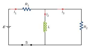
**59.** For the circuit shown below,  $\varepsilon = 50V, R_1 = 10\Omega, R_2 = R_3 = 19.4\Omega$  and L = 2.0mH. Find the values of  $I_1$  and  $I_2$
