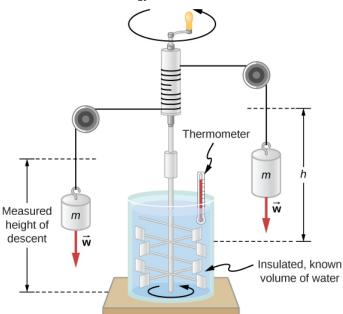
Figure 1.5.2: Joule's experiment established the equivalence of heat and work. As the masses descended, they caused the paddles to do work, W = mgh, on the water. The result was a temperature increase,  $\Delta T$ , measured by the thermometer. Joule found that  $\Delta T$  was proportional to **W** and thus determined the mechanical equivalent of heat.
