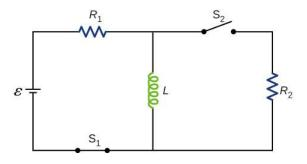
**54.** The current in the **RL** circuit shown here increases to **40%** of its steady-state value in 2.0 s. What is the time constant of the circuit?
