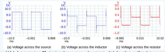
Figure 14.5.4: A generator in an **RL** circuit produces a square-pulse output in which the voltage oscillates between zero and some set value. These oscilloscope traces show (a) the voltage across the source; (b) the voltage across the inductor; (c) the voltage across the resistor.
