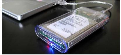
Figure 12.1.1: An external hard drive attached to a computer works by magnetically encoding information that can be stored or retrieved quickly. A key idea in the development of digital devices is the ability to produce and use magnetic fields in this way. (credit: modification of work by "Miss Karen"/Flickr)
