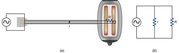
Figure 10.7.1: A short circuit is an undesired low-resistance path across a voltage source. (a) Worn insulation on the wires of a toaster allow them to come into contact with a low resistance **r**. Since  $P = V^2/\tau$ , thermal power is created so rapidly that the cord melts or burns. (b) A schematic of the short circuit.
