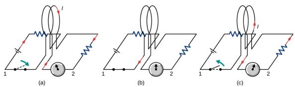
Figure 13.2.2: (a) Closing the switch of circuit 1 produces a short-lived current surge in circuit 2. (b) If the switch remains closed, no current is observed in circuit 2. (c) Opening the switch again produces a short-lived current in circuit 2 but in the opposite direction from before.
