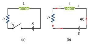
**57.** The current in the **RL** circuit shown below reaches half its maximum value in 1.75 ms after the switch  $S_1$  is thrown. Determine
