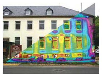
Figure 1.7.14: A thermograph of part of a building shows temperature variations, indicating where heat transfer to the outside is most severe. Windows are a major region of heat transfer to the outside of homes. (credit: US Army)
