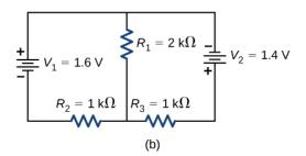
**38.** Consider the circuit shown below. Find  $V_1$ ,  $I_2$ , and  $I_3$ .
