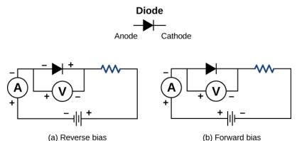
Figure 9.5.3: A diode is a semiconducting device that allows current flow only if the diode is forward biased, which means that the anode is positive and the cathode is negative.
