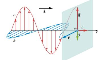
Figure 16.5.1: Electric and magnetic fields of an electromagnetic wave can combine to produce a force in the direction of propagation, as illustrated for the special case of electrons whose motion is highly damped by the resistance of a metal.
