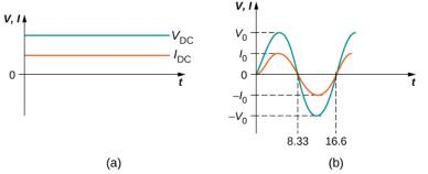
Figure 15.2.1: (a) The dc voltage and current are constant in time, once the current is established. (b) The voltage and current versus time are quite different for ac power. In this example, which shows 60-Hz ac power and time t in milliseconds, voltage and current are sinusoidal and are in phase for a simple resistance circuit. The frequencies and peak voltages of ac sources differ greatly.
