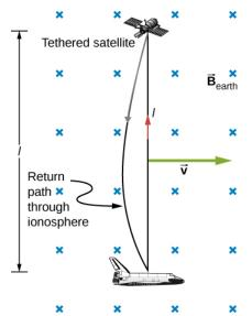
Figure 13.4.5: Motional emf as electrical power conversion for the space shuttle was the motivation for the tethered satellite experiment. A 5-kV emf was predicted to be induced in the 20-km tether while moving at orbital speed in Earth's magnetic field. The circuit is completed by a return path through the stationary ionosphere.
