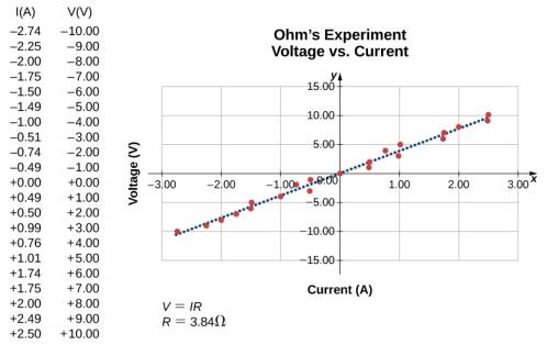
Figure 9.5.1: A resistor is placed in a circuit with a battery. The voltage applied varies from -10.00 V to +10.00 V, increased by 1.00-V increments. A plot shows values of the voltage versus the current typical of what a casual experimenter might find.
