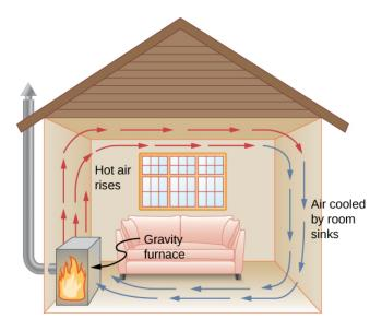
Figure 1.7.6: Air heated by a so-called gravity furnace expands and rises, forming a convective loop that transfers energy to other parts of the room. As the air is cooled at the ceiling and outside walls, it contracts, eventually becoming denser than room air and sinking to the floor. A properly designed heating system using natural convection, like this one, can heat a home quite efficiently.
