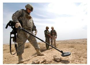
Figure 13.6.6: A soldier in Iraq uses a metal detector to search for explosives and weapons. (credit: U.S. Army)
