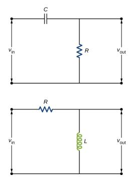
**72.** The two circuits shown below act as crude low-pass filters. The input voltage to the circuits is  $v_{in}$ , and the output voltage is  $v_{out}$ .
