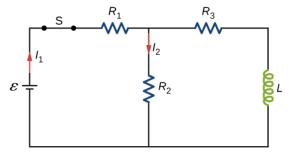
**61.** Show that for the circuit shown below, the initial energy stored in the inductor,  $LI^2(0)/2$ , is equal to the total energy eventually dissipated in the resistor,  $\int_0^\infty I^2(t)Rdt$ .
