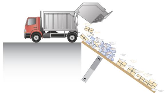
Figure 13.6.5: Metals can be separated from other trash by magnetic drag. Eddy currents and magnetic drag are created in the metals sent down this ramp by the powerful magnet beneath it. Nonmetals move on.
