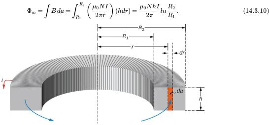
Figure 14.3.6: Calculating the self-inductance of a rectangular toroid.
