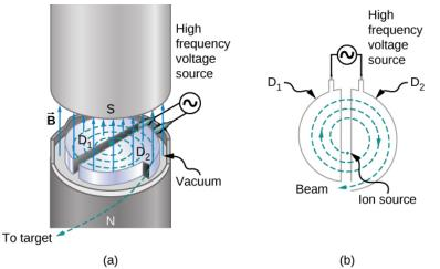
Figure 11.8.2: The inside of a cyclotron. A uniform magnetic field is applied as circulating protons travel through the dees, gaining energy as they traverse through the gap between the dees.
