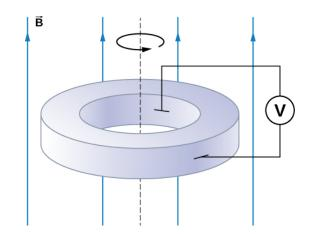
**85.** A long solenoid with 10 turns per centimeter is placed inside a copper ring such that both objects have the same central axis. The radius of the ring is 10.0 cm, and the radius of the solenoid is 5.0 cm.
