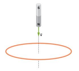
**13.** The accompanying figure shows a conducting ring at various positions as it moves through a magnetic field. What is the sense of the induced emf for each of those positions?
