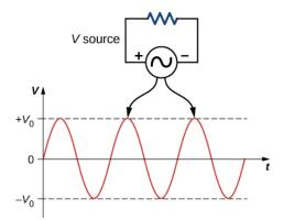
Figure 15.2.2: The potential difference **V** between the terminals of an ac voltage source fluctuates, so the source and the resistor have ac sine waves on top of each other. The mathematical expression for **v** is given by  $v = V_0 \sin \omega t$ .
