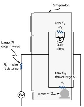
Figure 10.3.7: Why do lights dim when a large appliance is switched on? The answer is that the large current the appliance motor draws causes a significant **IR** drop in the wires and reduces the voltage across the light.
