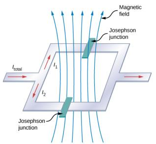
Figure 9.7.3: The SQUID (superconducting quantum interference device) uses a superconducting current loop and two Josephson junctions to detect magnetic fields as low as  $10^{-14}$  (Earth's magnet field is on the order of  $0.3 \times 10^{-5}T$ ).
