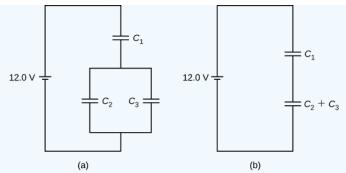
Figure 8.3.4: (a) A capacitor combination. (b) An equivalent two-capacitor combination.
