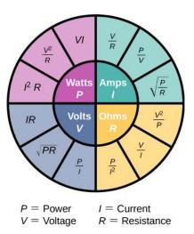
Figure 9.6.4: This circle shows a summary of the equations for the relationships between power, current, voltage, and resistance.
