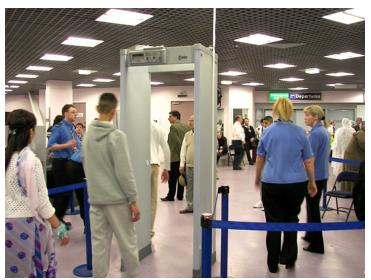
Figure 14.3.5: The familiar security gate at an airport not only detects metals, but can also indicate their approximate height above the floor. (credit: "Alexbuirds"/Wikimedia Commons)
