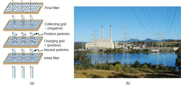
Figure 7.7.5: (a) Schematic of an electrostatic precipitator. Air is passed through grids of opposite charge. The first grid charges airborne particles, while the second attracts and collects them. (b) The dramatic effect of electrostatic precipitators is seen by the absence of smoke from this power plant. (credit b: modification of work by "Cmdalgleish"/Wikimedia Commons)
