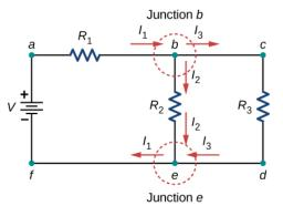
Figure 10.4.6: At first glance, this circuit contains two junctions, Junction  $\mathbf{b}$  and Junction  $\mathbf{e}$ , but only one should be considered because their junction equations are equivalent.
