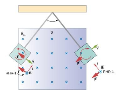
Figure 13.6.2: A more detailed look at the conducting plate passing between the poles of a magnet. As it enters and leaves the field, the change in flux produces an eddy current. Magnetic force on the current loop opposes the motion. There is no current and no magnetic drag when the plate is completely inside the uniform field.
