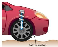
Figure 15.4.5: On a car, the shock absorber damps motion and dissipates energy. This is much like the resistance in an RLC circuit. The mass and spring determine the resonant frequency.
