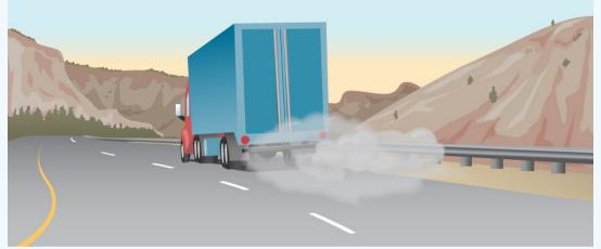
Figure 1.5.3: The smoking brakes on a braking truck are visible evidence of the mechanical equivalent of heat.
