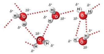
Figure 16.6.3: The oscillating electric field in a microwave oven exerts a torque on water molecules because of their dipole moment, and the torque reverses direction  $4.90 \times 10^9$  times per second. Interactions between the molecules distributes the energy being pumped into them. The  $\delta^+$  and  $\delta^-$  denote the charge distribution on the molecules.
