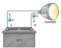
Figure 7.3.1: A battery moves negative charge from its negative terminal through a headlight to its positive terminal. Appropriate combinations of chemicals in the battery separate charges so that the negative terminal has an excess of negative charge, which is repelled by it and attracted to the excess positive charge on the other terminal. In terms of potential, the positive terminal is at a higher voltage than the negative terminal. Inside the battery, both positive and negative charges move.
