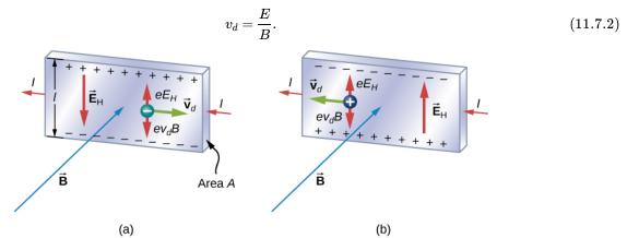
Figure 11.7.1: In the Hall effect, a potential difference between the top and bottom edges of the metal strip is produced when moving charge carriers are deflected by the magnetic field. (a) Hall effect for negative charge carriers; (b) Hall effect for positive charge carriers.
