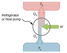
Figure 4.4.1: A schematic representation of a refrigerator (or a heat pump). The arrow next to work (W) indicates work being put into the system.
