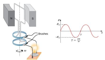
Figure 13.7.3: The emf of a generator is sent to a light bulb with the system of rings and brushes shown. The graph gives the emf of the generator as a function of time, where  $\epsilon_0$  is the peak emf. The period is  $T = 1/f = 2\pi/\omega$ , where **f** is the frequency.
