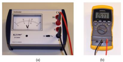
Figure 10.5.4: (a) An analog voltmeter uses a galvanometer to measure the voltage. (b) Digital meters use an analog-to-digital converter to measure the voltage. (credit a and credit b: Joseph J. Trout)
