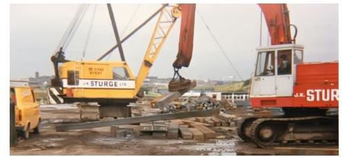
Figure 11.1.1: An industrial electromagnet is capable of lifting thousands of pounds of metallic waste. (credit: modification of work by "BedfordAl"/Flickr)
