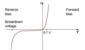
Figure 9.5.4: When the voltage across the diode is negative and small, there is very little current flow through the diode. As the voltage reaches the breakdown voltage, the diode conducts. When the voltage across the diode is positive and greater than 0.7 V (the actual voltage value depends on the diode), the diode conducts. As the voltage applied increases, the current through the diode increases, but the voltage across the diode remains approximately 0.7 V.
