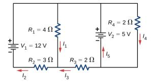
42. Consider the circuit shown below. Write the three loop equations for the loops shown.
