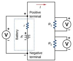
Figure 10.5.3: To measure potential differences in this series circuit, the voltmeter (V) is placed in parallel with the voltage source or either of the resistors. Note that terminal voltage is measured between the positive terminal and the negative terminal of the battery or voltage source. It is not possible to connect a voltmeter directly across the emf without including the internal resistance  $\mathbf{r}$  of the battery.
