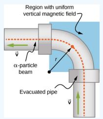
Figure 11.4.4: Top view of the beam deflector setup.
