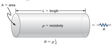
Figure 9.4.3: A model of a resistor as a uniform cylinder of length **L** and cross-sectional area **A**. Its resistance to the flow of current is analogous to the resistance posed by a pipe to fluid flow. The longer the cylinder, the greater its resistance. The larger its cross-sectional area **A**, the smaller its resistance.
