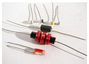
Figure 14.3.3: A variety of inductors. Whether they are encapsulated like the top three shown or wound around in a coil like the bottom-most one, each is simply a relatively long coil of wire. (credit: Windell Oskay)
