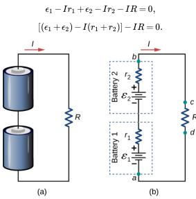
Figure 10.4.13: (a) Two batteries connected in series with a load resistor. (b) The circuit diagram of the two batteries and the load resistor, with each battery modeled as an idealized emf source and an internal resistance.
