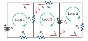
43. Consider the circuit shown below. Write equations for the three currents in terms of R and V.
