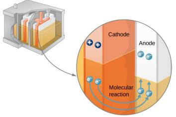
Figure 10.2.4: In a lead-acid battery, two electrons are forced onto the anode of a cell, and two electrons are removed from the cathode of the cell. The chemical reaction in a lead-acid battery places two electrons on the anode and removes two from the cathode. It requires a closed circuit to proceed, since the two electrons must be supplied to the cathode.
