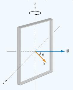
Figure 13.4.7: A rectangular coil rotating in a uniform magnetic field.
