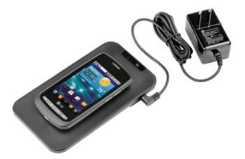
Figure 14.1.1: A smartphone charging mat contains a coil that receives alternating current, or current that is constantly increasing and decreasing. The varying current induces an emf in the smartphone, which charges its battery. Note that the black box containing the electrical plug also contains a transformer (discussed in Alternating-Current Circuits) that modifies the current from the outlet to suit the needs of the smartphone. (credit: modification of work by "LG"/Flickr)
