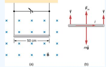
Figure 11.5.3: (a) A wire suspended in a magnetic field. (b) The free-body diagram for the wire.
