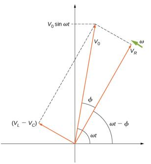
Figure 15.4.3: The resultant of the phasors for  $v_L(t)$ ,  $v_C(t)$ , and  $v_R(t)$  is equal to the phasor for  $v_R(t) = V_0 \sin \omega t$ . The **i**(**t**) phasor (not shown) is aligned with the  $v_R(t)$  phasor.
