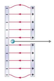
Figure 7.9.1: Parallel conducting plates with opposite charges on them create a relatively uniform electric field used to accelerate electrons to the right. Those that go through the hole can be used to make a TV or computer screen glow or to produce X-rays.
