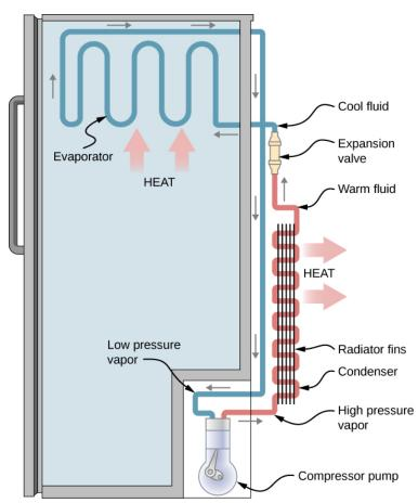
Figure 4.4.2: A schematic diagram of a household refrigerator. A coolant with a boiling temperature below the freezing point of water is sent through the cycle (clockwise in this diagram). The coolant extracts heat from the refrigerator at the evaporator, causing coolant to vaporize. It is then compressed and sent through the condenser, where it exhausts heat to the outside.
