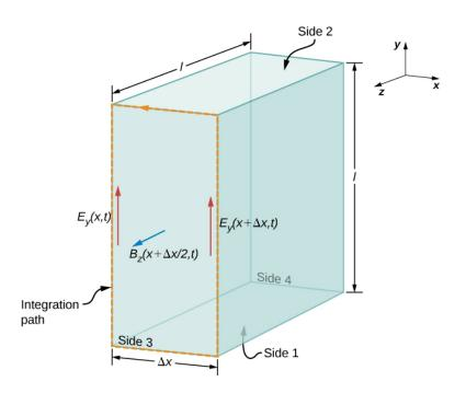
Figure 16.3.2: We apply Faraday's law to the front of the rectangle by evaluating  $\oint \vec{E} \cdot d\vec{s}$  along the rectangular edge of Side 3 in the direction indicated, taking the B field crossing the face to be approximately its value in the middle of the area traversed.
