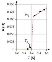
Figure 9.7.1: The resistance of a sample of mercury is zero at very low temperatures—it is a superconductor up to the temperature of about 4.2 K. Above that critical temperature, its resistance makes a sudden jump and then increases nearly linearly with temperature.
