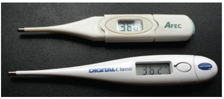
Figure 9.4.5: These familiar thermometers are based on the automated measurement of a thermistor's temperature-dependent resistance.
