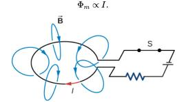
Figure 14.3.1: A magnetic field is produced by the current **I** in the loop. If **I** were to vary with time, the magnetic flux through the loop would also vary and an emf would be induced in the loop.
