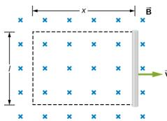
Figure 13.4.4: With the imaginary rectangle shown, we can use Faraday's law to calculate the induced emf in the moving rod.
