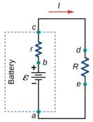
Figure 10.2.6: Schematic of a voltage source and its load resistor **R**. Since the internal resistance **r** is in series with the load, it can significantly affect the terminal voltage and the current delivered to the load.
