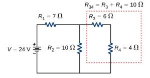
(b) Step 1: resistors R<sub>3</sub> and R<sub>4</sub> in series
