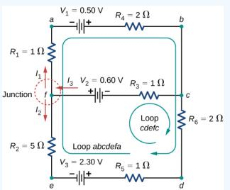
Figure 10.4.11: This circuit is combination of series and parallel configurations of resistors and voltage sources. This circuit cannot be analyzed using the techniques discussed in <u>Electromotive Force</u> but can be analyzed using Kirchhoff's rules.
