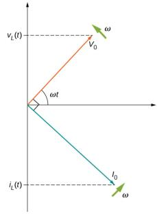
Figure 15.3.7: The current phasor lags the voltage phasor by  $\pi/2$  rad as they both rotate with the same angular frequency.
