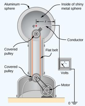
Figure 7.4.1: The voltage of this demonstration Van de Graaff generator is measured between the charged sphere and ground. Earth's potential is taken to be zero as a reference. The potential of the charged conducting sphere is the same as that of an equal point charge at its center.
