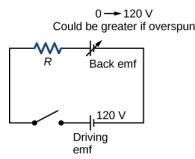
Figure 13.7.6: The coil of a dc motor is represented as a resistor in this schematic. The back emf is represented as a variable emf that opposes the emf driving the motor. Back emf is zero when the motor is not turning and increases proportionally to the motor's angular velocity.
