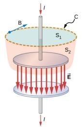
Figure 16.2.2: The currents through surface  $S_1$  and surface  $S_2$  are unequal, despite having the same boundary loop C.
