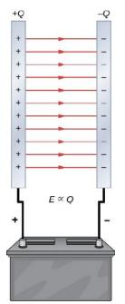
Figure 8.2.2: The charge separation in a capacitor shows that the charges remain on the surfaces of the capacitor plates. Electrical field lines in a parallel-plate capacitor begin with positive charges and end with negative charges. The magnitude of the electrical field in the space between the plates is in direct proportion to the amount of charge on the capacitor.
