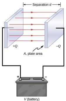
Figure 8.2.4: In a parallel-plate capacitor with plates separated by a distance (d), each plate has the same surface area (A). We define the surface charge density  $\sigma$  on the plates as
