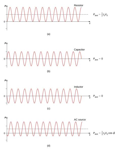
Figure 15.5.1: Graph of instantaneous power for various circuit elements. (a) For the resistor,  $P_{ave} = I_0 V_0/2$ , whereas for (b) the capacitor and (c) the inductor,  $P_{ave} = 0$ . (d) For the source,  $P_{ave} = I_0 V_0(\cos \phi)/2$ , which may be positive, negative, or zero, depending on  $\phi$ .
