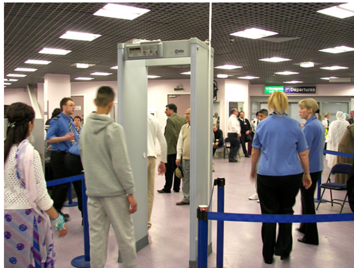
Figure 14.3.5: The familiar security gate at an airport not only detects metals, but can also indicate their approximate height above the floor. (credit: "Alexbuidrds"/Wikimedia Commons)
