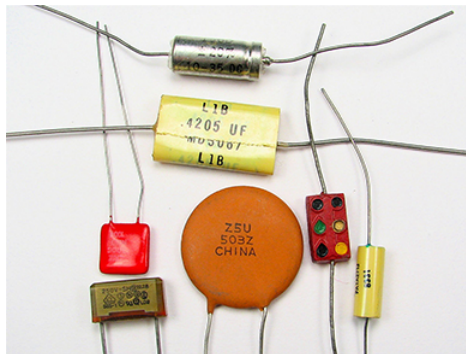
Figure 8.2.3: These are some typical capacitors used in electronic devices. A capacitor's size is not necessarily related to its capacitance value.
