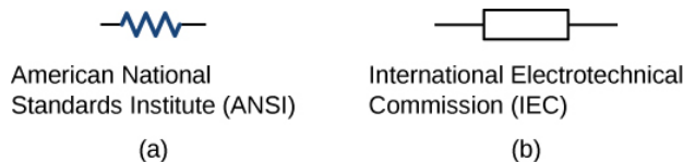
Figure 9.4.2: Symbols for a resistor used in circuit diagrams. (a) The ANSI symbol; (b) the IEC symbol.
