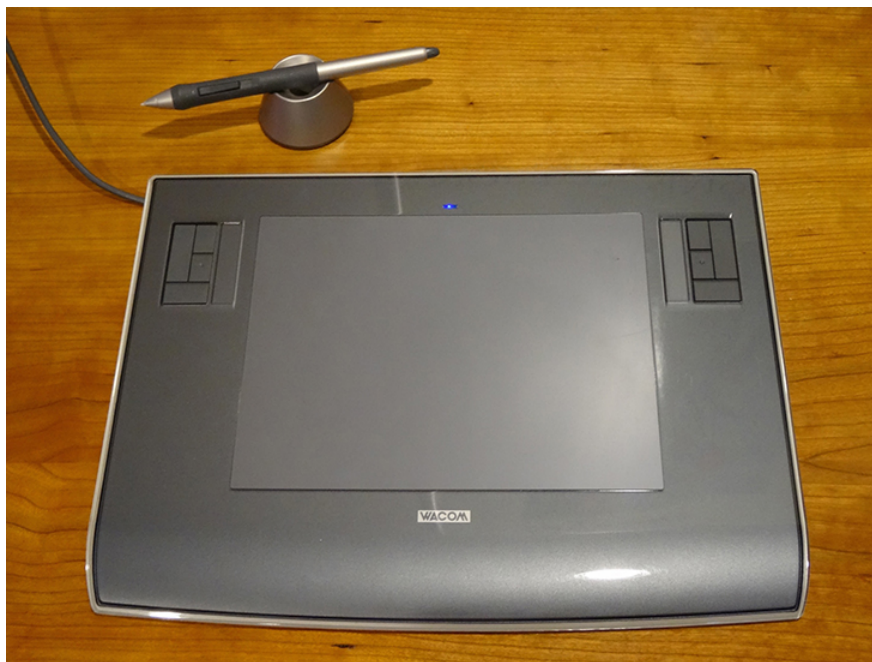
Figure 13.8.1: A tablet with a specially designed pen to write with is another application of magnetic induction.
