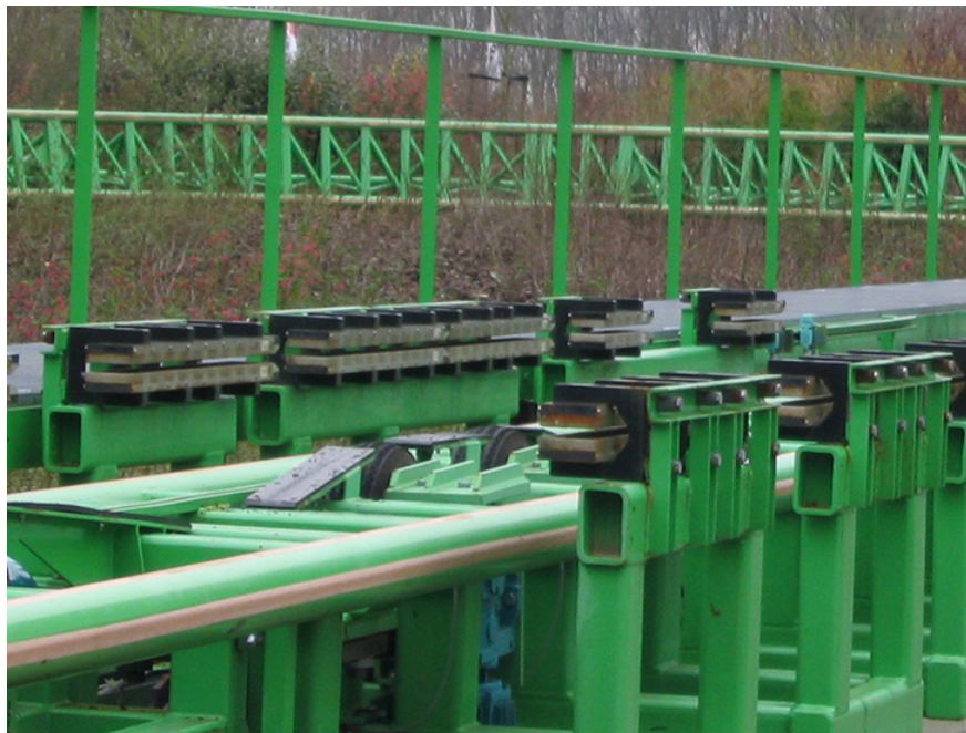
Figure 13.6.7: The rows of rare-earth magnets (protruding horizontally) are used for magnetic braking in roller coasters. (credit: Stefan Scheer)
