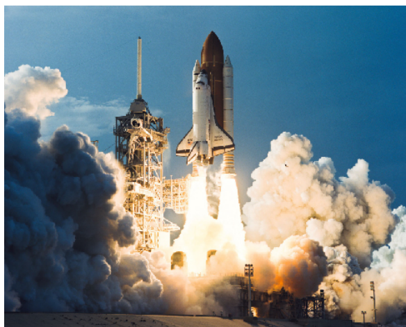
Figure 2.5.2 Demonstrating Newton's Third Law. The U.S. Space Shuttle (here launching Discovery), powered by three fuel engines burning liquid oxygen and liquid hydrogen, with two solid fuel boosters, demonstrates Newton's third law. (credit: modification of work by NASA)
