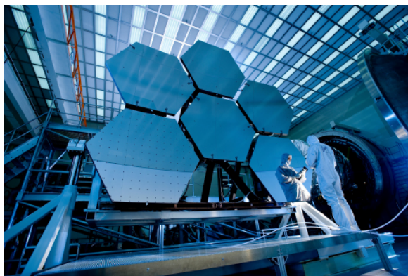
Figure 3.12.1 James Webb Space Telescope (JWST). This image shows some of the mirrors of the JWST as they underwent cryogenic testing. The mirrors were exposed to extreme temperatures in order to gather accurate measurements on changes in their shape as they heated and cooled. (credit: NASA/MSFC/David Higginbotham/Emmett Given)
