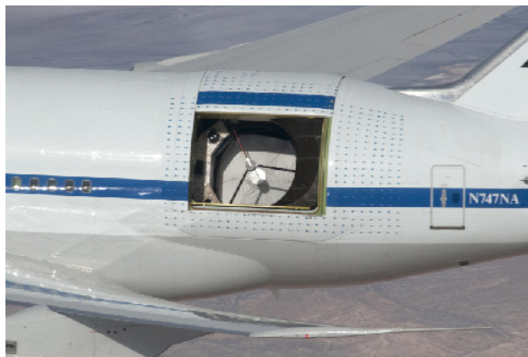
Figure 3.11.1 Stratospheric Observatory for Infrared Astronomy (SOFIA). SOFIA allows observations to be made above most of Earth's atmospheric water vapor.
